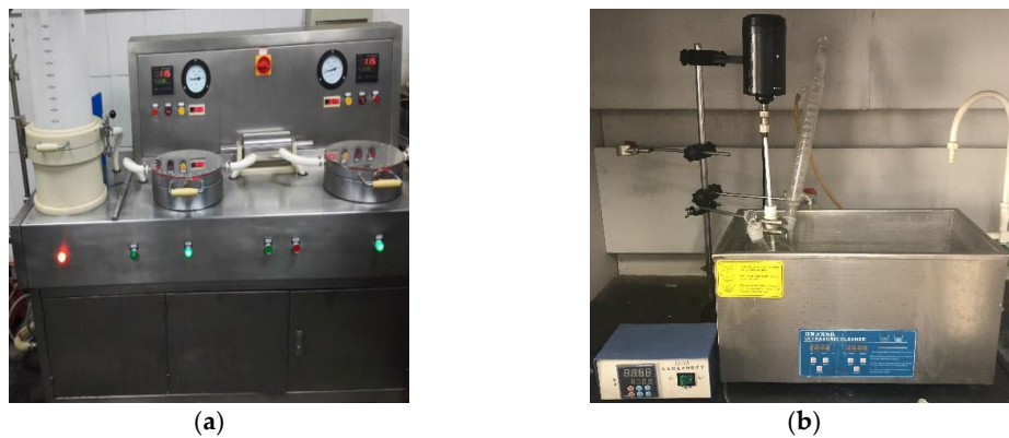
Figure 1. (a) Fast paper sheet former; (b) Nano-Al 2 O 3 surface treatment.
