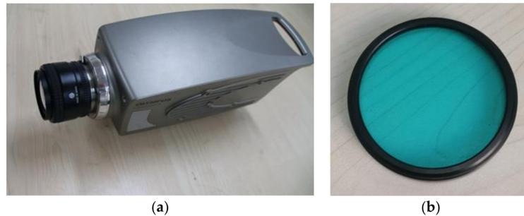
**Figure 5.** Flame measuring instruments: (a) high-speed camera; (b) optical filter.
