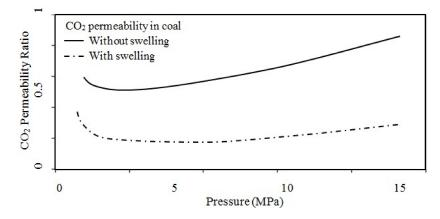
Figure 3. Change of CO<sub>2</sub> permeability in coal with swelling process and the pressure effect on it [34].
