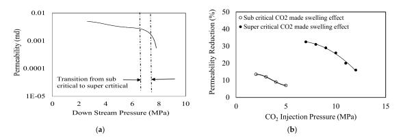
**Figure 10.** Variation of coal permeability with pore pressure for both sub-critical and super- critical CO<sub>2</sub>. (a) Down Stream Pressure [3]; (b) CO<sub>2</sub> Injection Pressure [54].
