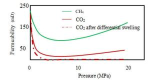
Figure 16. Differential swelling during CO<sub>2</sub> flow in coal [51].
