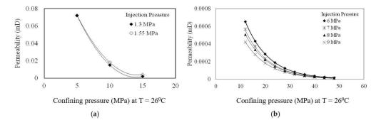
**Figure 7.** Influence of confining stress on CO<sub>2</sub> permeability in (**a**) Indian [40], and, (**b**) Australian [48] bituminous coals.
