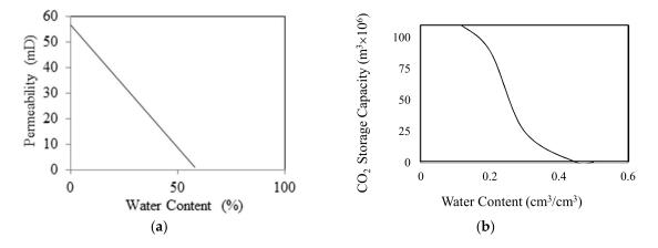
**Figure 1.** Variation of coal seam permeability (**a**) [20], and gas storage capacity (**b**) [21] with natural moisture content.
