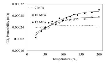
**Figure 13.** Influence of temperature on  $CO_2$  flow ability in bituminous coal for various  $CO_2$  pressures [23].
