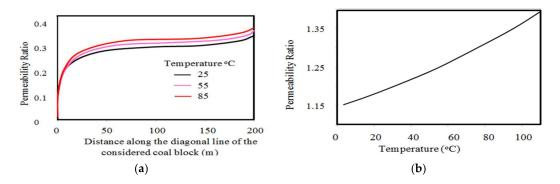
**Figure 14.** Influence of temperature on CO<sub>2</sub> flow ability in coal at various CO<sub>2</sub> injection pressures [62]. (a) 7 MPa CO<sub>2</sub> injection pressure; (b) 10 MPa CO<sub>2</sub> injection pressure.
