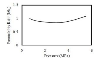
Figure 8. Variation of coal permeability with pore pressure [52].
