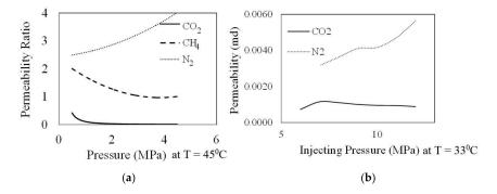
**Figure 5.** Unique flow behaviour of CO<sub>2</sub> in coal observed by different researchers. (**a**) Durucan and Shi [35]; (**b**) Perera et al. [3].
