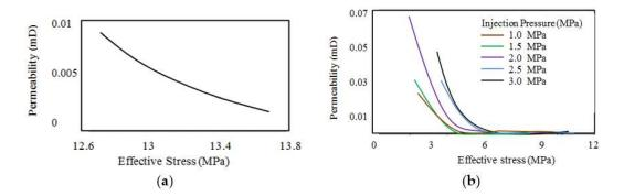
**Figure 12.** Influence of effective stress on CO<sub>2</sub> permeability in (**a**) high-rank coal [40], and (**b**) low-rank coal [36].
