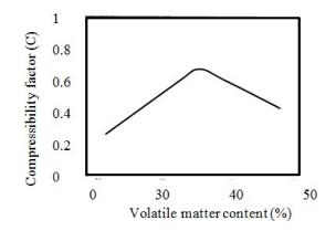
Figure 15. Volatile matter content-dependent compressibility factor of coal [19].
