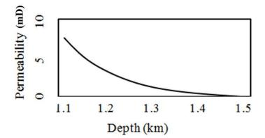
Figure 2. Variation of coal permeability with seam location [30].
