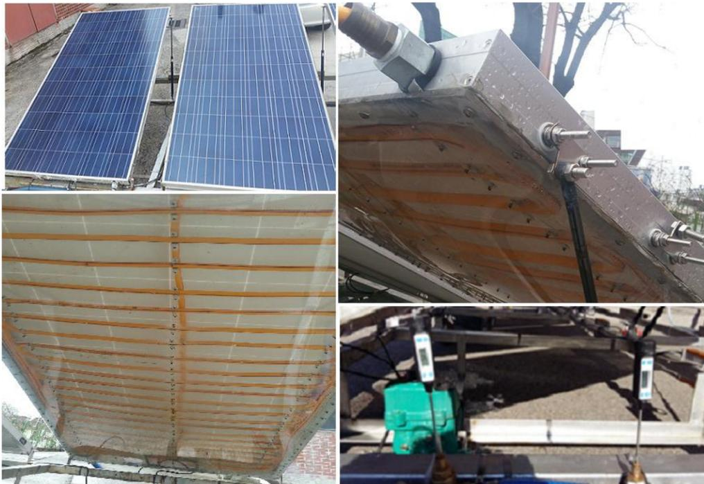
**Figure 8.** Experimental setup for proposed closed-loop cooled solar system (CLC-SS).
