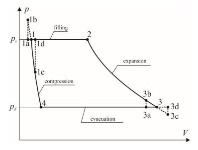
Figure 7. The multi-vane expander indicator diagram.
