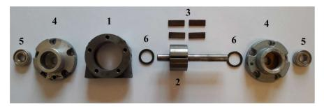
**Figure 1.** A general view of the expander. (1) cylinder; (2) rotor; (3) vanes; (4) end covers; (5) rolling bearings; (6) rings.
