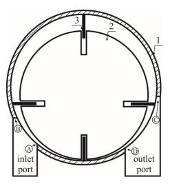
Figure 6. The cross section of the multi-vane expander at  $0^{\circ}$  crank angle. (1) cylinder; (2) rotor; (3) vane.
