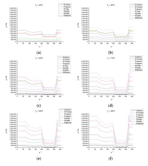
**Figure 3.** Pressure distribution against crank angle for different working fluids and inlet temperatures: (a)  $t_{in} = 40 \degree C$ ; (b)  $t_{in} = 50 \degree C$ ; (c)  $t_{in} = 60 \degree C$ ; (d)  $t_{in} = 70 \degree C$ ; (e)  $t_{in} = 80 \degree C$ ; (f)  $t_{in} = 90 \degree C$ .
