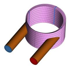
**Figure 2.** The initial position of the numerical mesh of the computational model at crank angle  $\phi = 0^{\circ}$ . The working fluid flow was modelled as a compressible, turbulent, and single-phase Redlich–Kwong gas. The specific heat capacity of each tested medium was set as a function of temperature. The wall boundary was assumed adiabatic due to the brief time spent by a portion of the fluid inside the machine (see Table 1).
