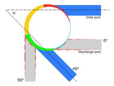
**Figure 8.** The modified multi-vane expander's construction with different locations of machine steering edges ( $\alpha = 0^{\circ}$ , 22.5°, 45°, 67.5°, and 90°).
