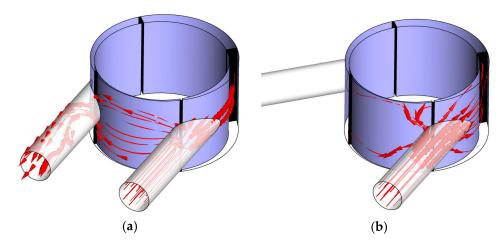
**Figure 14.** The visualization of leakage from the inlet to the outlet port of the expander: (**a**) present design; (**b**) improved design.
