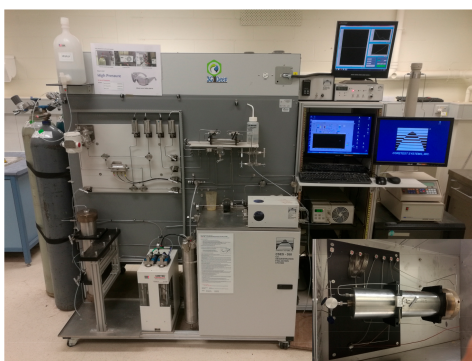
Figure 2. Core flooding set-up for permeability tests.
