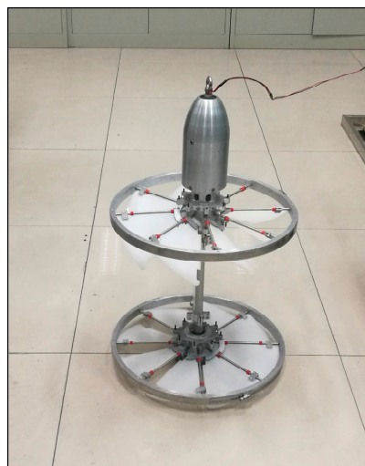
Figure 18. WEC physical prototype. WEC: wave energy converter.
