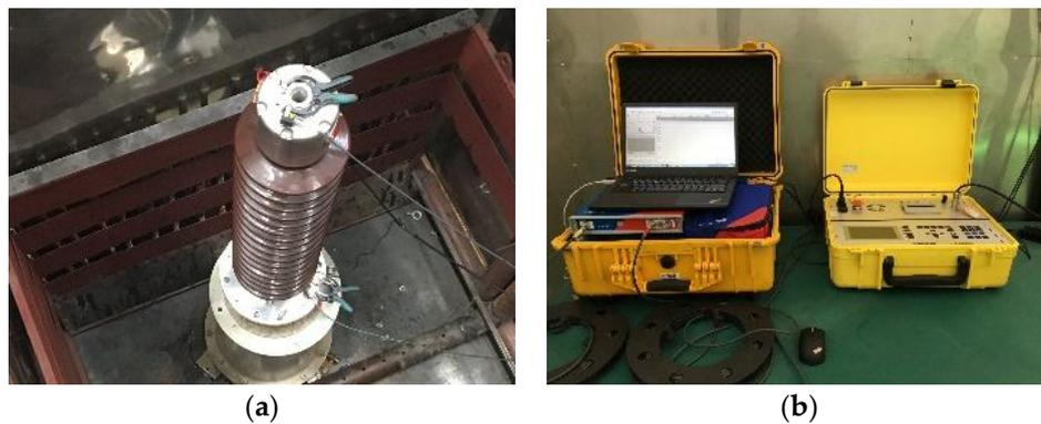
**Figure 4.** (a) OIP condenser bushing placed in an oast house for tests; (b) dielectric response analyzer and recovery voltage meter.
