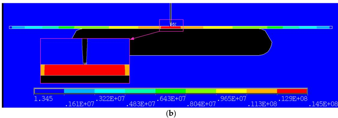
**Figure 7.** Electric field distribution of needle-plate model under AC and DC voltage components. (a) AC voltage component; (b) DC voltage component.
