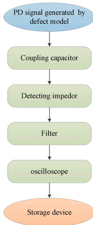
Figure 4. Flow diagram of the PD measurement.
