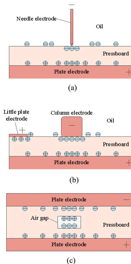
**Figure 8.** Space charge distribution diagram under DC component. (a) Needle-plate; (b) Surface discharge; (c) Air gap.
