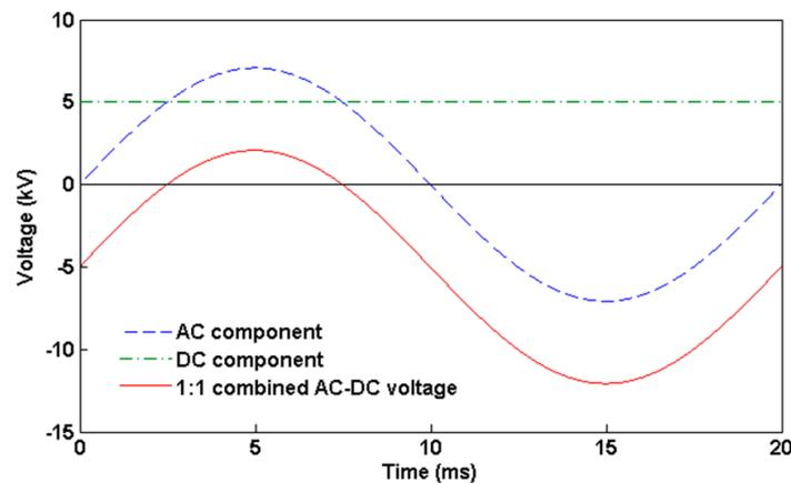
Figure 3. The applied voltage waveform.
