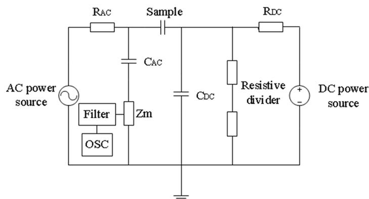
Figure 1. Schematic diagram of the experimental arrangement.
