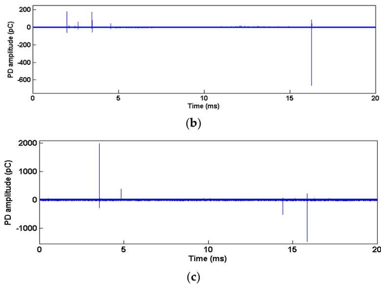
**Figure 6.** PD pulses in one primitive cycle of three models. (a) Needle-plate; (b) Surface discharge; (c) Air gap.
