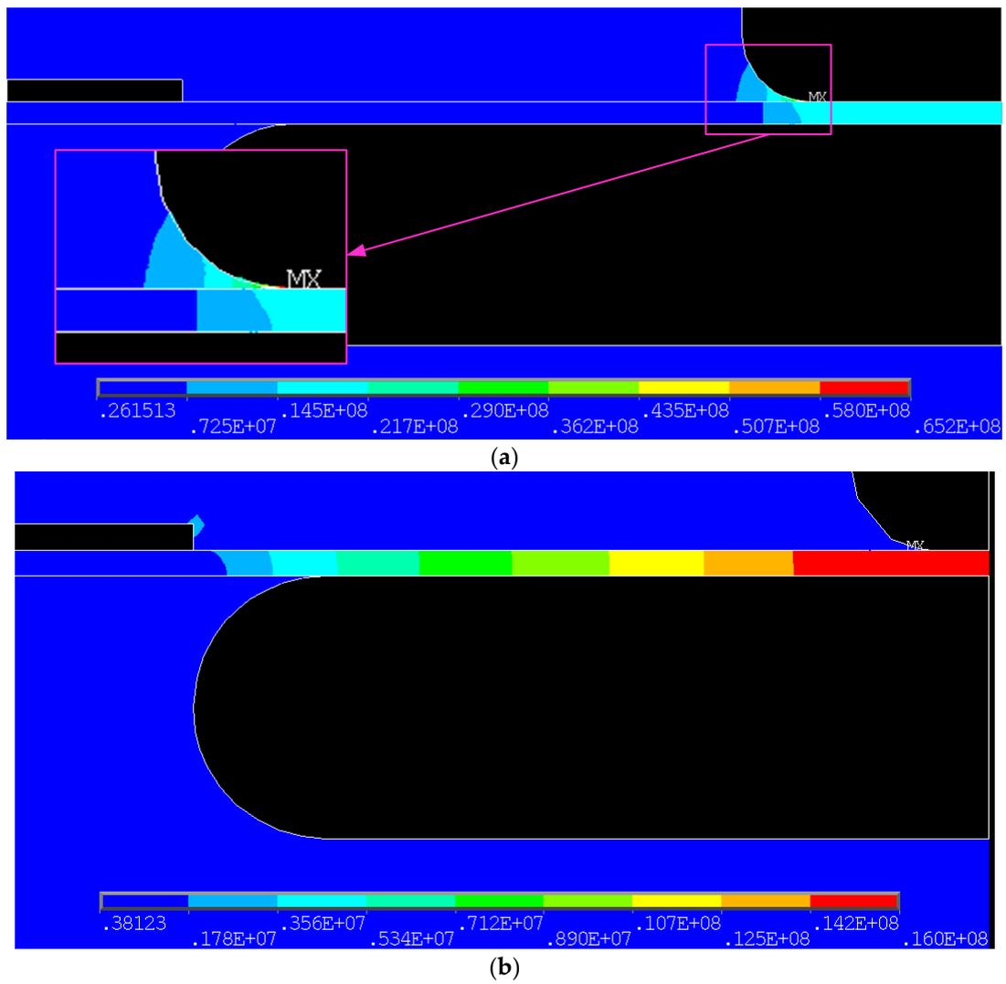
**Figure 9.** Electric field distribution of surface discharge model under AC and DC voltage components. (a) AC voltage component; (b) DC voltage component.
