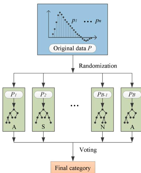
**Figure 11.** Flowchart of PD source type classification with RF.
