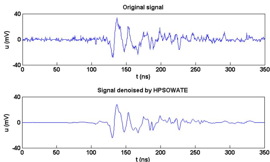
**Figure 12.** Original signal and de-noised signal of oscillation-attenuated PD pulse.
