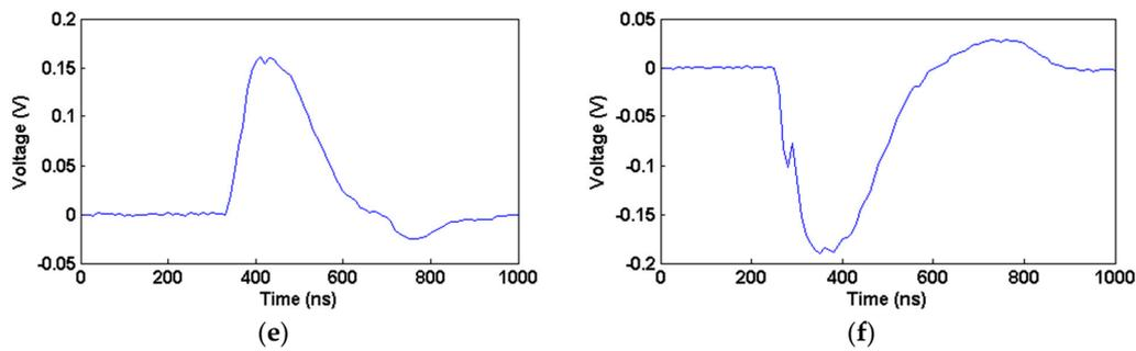
**Figure 13.** Single PD pulses of three models. (a) Positive half cycle of needle-plate; (b) Negative half cycle of needle-plate; (c) Positive half cycle of surface discharge; (d) Negative half cycle of surface discharge; (e) Positive half cycle of air gap; (f) Negative half cycle of air gap.
