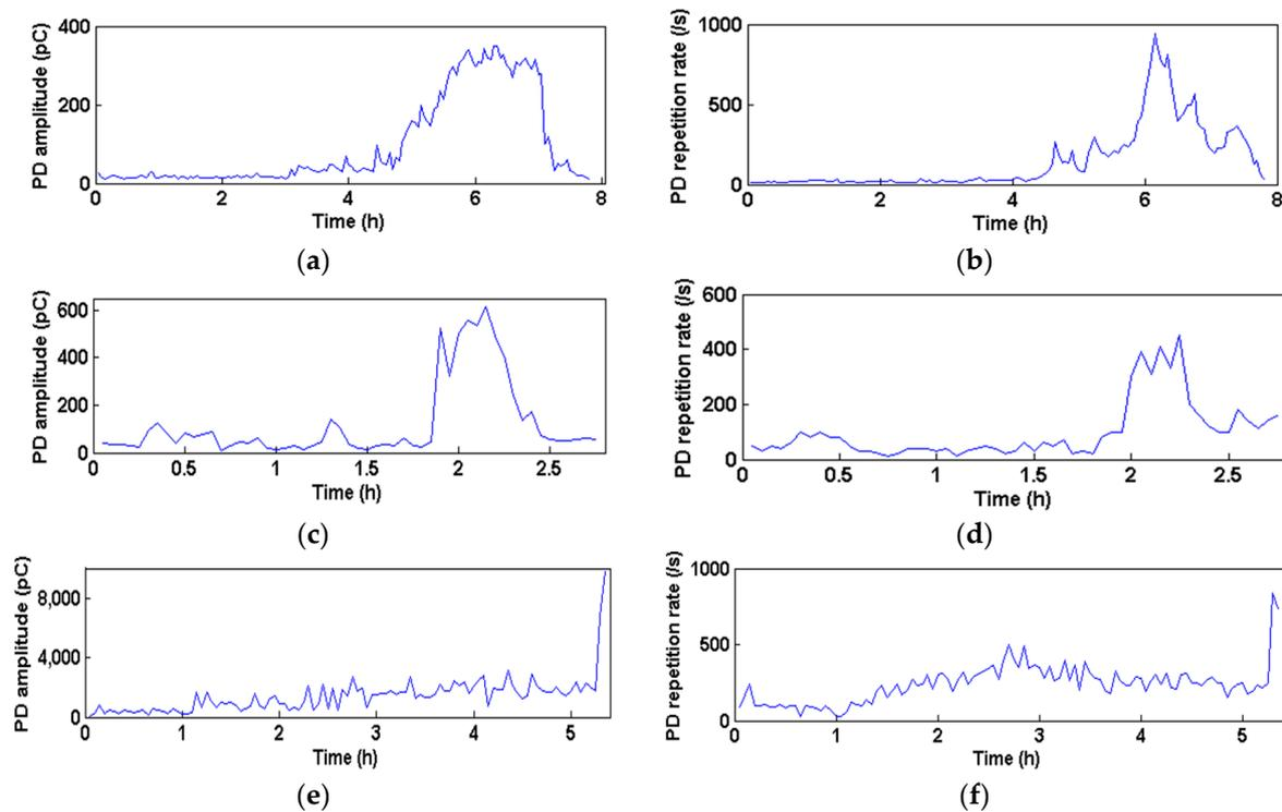
**Figure 5.** Time-variation trends of  $Q_{\max}$  and  $N$  of three models. (a)  $Q_{\max}$  of needle-plate; (b)  $N$  of needle-plate; (c)  $Q_{\max}$  of surface discharge; (d)  $N$  of surface discharge; (e)  $Q_{\max}$  of air gap; (f)  $N$  of air gap.
