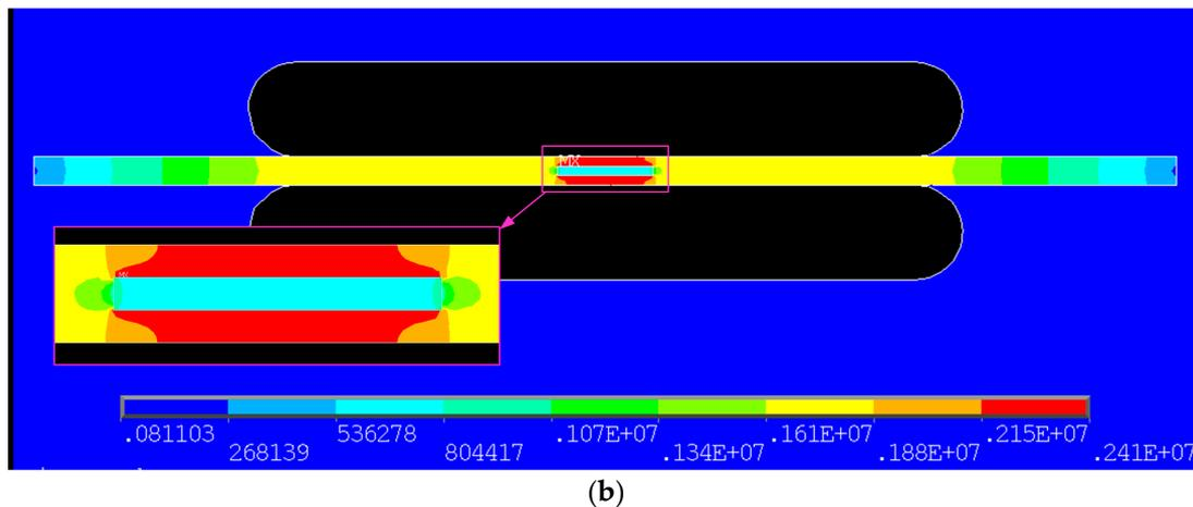
**Figure 10.** Electric field distribution of air gap model under AC and DC voltage components. (a) AC voltage component; (b) DC voltage component.
