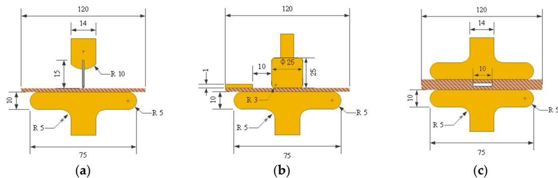
**Figure 2.** Schematic diagram of the electrodes. (a) Needle-plate; (b) Surface discharge; (c) Air gap.
