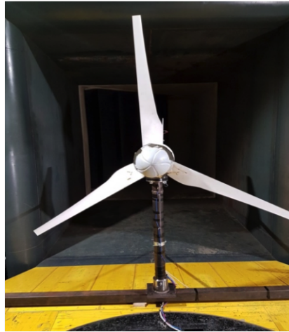
Figure 1. The front view of the wind turbine in the wind tunnel with the recovery test section ( 2.7 \text{ m} \times 2.7 \text{ m} ) on the background.
