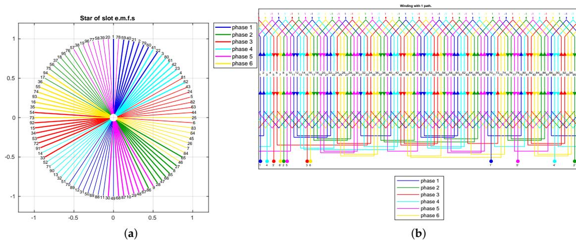
**Figure 18.** (a) Star of slots of a 6-phase reduced single-layer winding with  $N = 96$ ,  $p = 5$  and (b) related winding scheme with 1-st order double sided imbrication.
