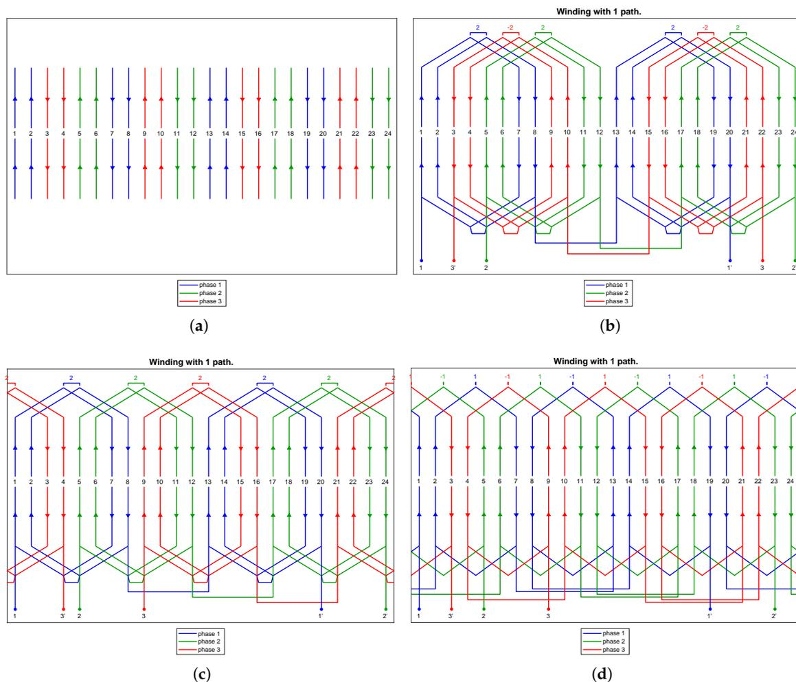
**Figure 2.** Winding schemes with different end winding layouts for a single-layer configuration with  $N = 24$ ,  $m = 3$ ,  $p = 2$  and  $q = 2$  derived from the WDT. (a) Without end connections; (b) for a split stator and three-plane end winding; (c) with two-plane end winding and (d) with three-plane end winding.
