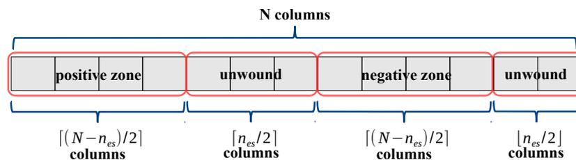
Figure 5. A possible WDT for single phase windings.
