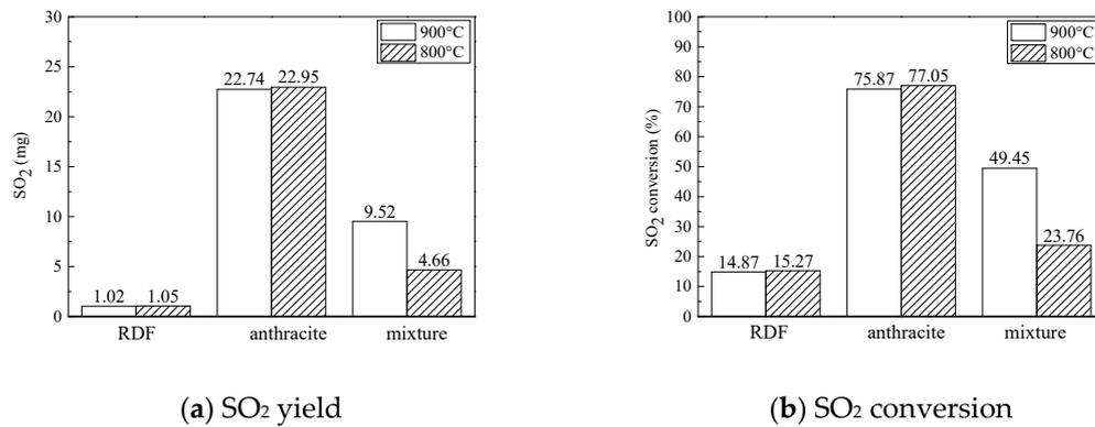
Figure 9. SO<sub>2</sub> emission yield and SO<sub>2</sub> conversion at different temperatures.
