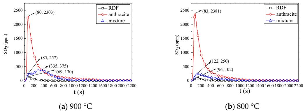
Figure 8. SO<sub>2</sub> emission curves at different temperatures.
