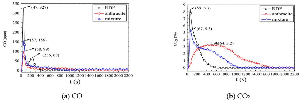
Figure 3. CO and CO<sub>2</sub> emission curves at 900 °C during combustion.
