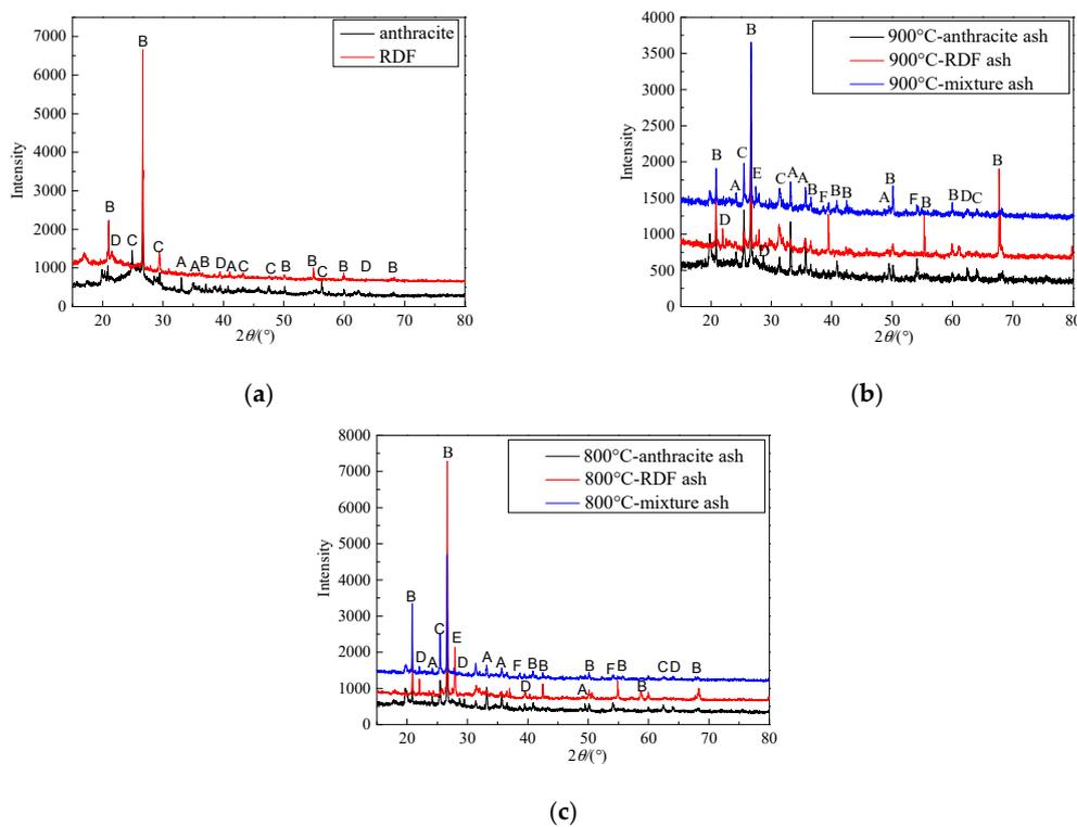
Figure 10. XRD analysis of fuels and different ashes: (a) original fuels; (b) ash at 900 °C; (c) ash at 800 °C, A-Fe<sub>2</sub>O<sub>3</sub>, B-SiO<sub>2</sub>, C-CaSO<sub>4</sub>, D-CaCO<sub>3</sub>, E-CaAl<sub>2</sub>Si<sub>2</sub>O<sub>8</sub>, and F-CaO.
