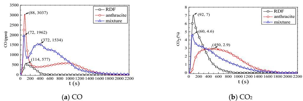
Figure 4. CO and CO<sub>2</sub> emission curves at 800 °C during combustion.
