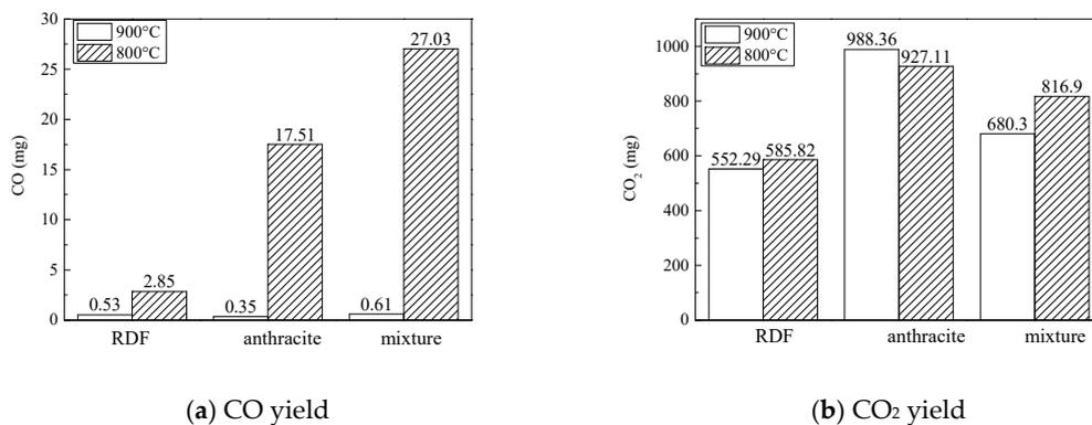
Figure 5. CO and CO<sub>2</sub> emission yield at different temperatures.
