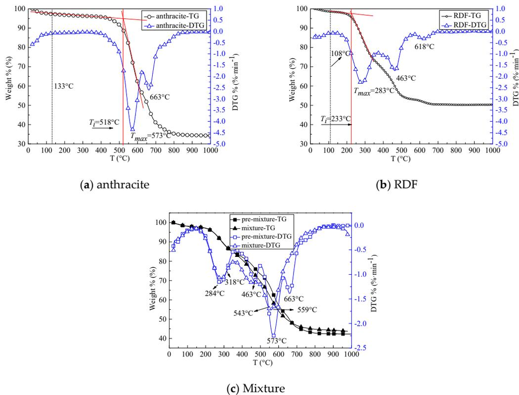
Figure 2. TG-DTG profiles of fuels combustion.
