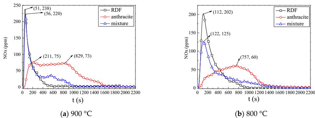
Figure 6. NOx emission curves at different temperatures.
