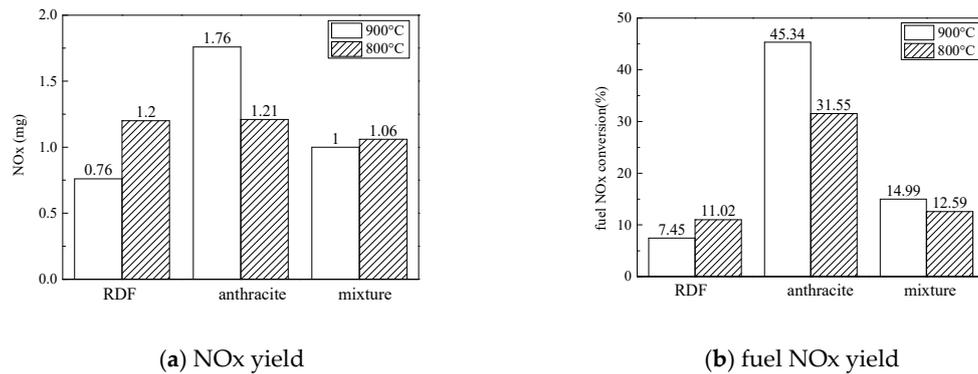
**Figure 7.** NOx emission yield and fuel NOx conversion at different temperatures.
