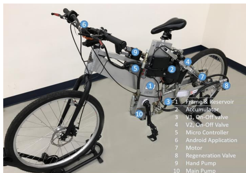
Figure 1. Physical design for PurdueTracer.
