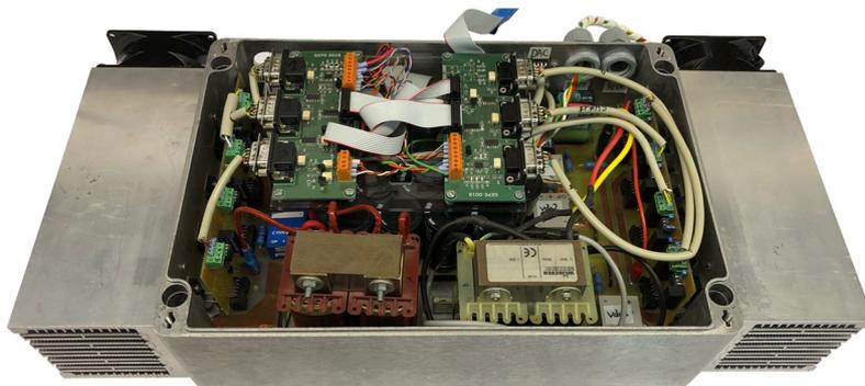
Figure 9. Laboratorial prototype of the developed EVBC.
