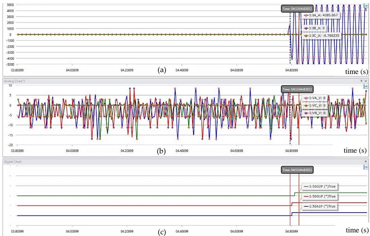
**Figure 8.** Fault waveforms and tripping signals corresponding to the SPGF at F1: (a) three phase currents (Ia (A), Ib (A), and Ic (A)); (b) three phase voltages (Va (V), Vb (C), and Vc (V)); (c) tripping signals of the ground OC relay (50G1P and 50G2P are two tripping signals of the ground OC relay at levels 1 and 2, respectively, while the 50A1P shows a faulted phase-A).
