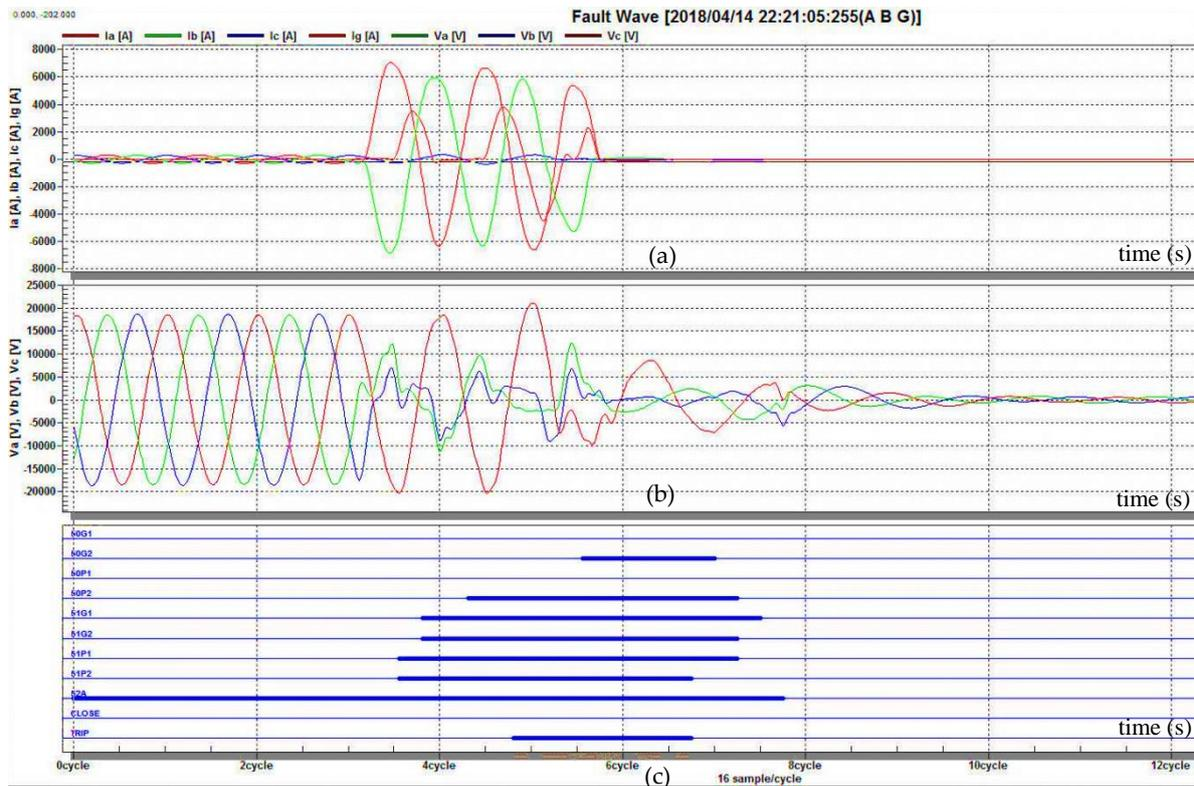
Figure 9. DPGF waveforms at the 473 Go-Noi feeder: (a) three phase currents Ia (A), Ib (A), Ic (A) and ground current Ig (A); (b) three phase voltages (Va (V), Vb (V), and Vc (V)); (c) tripping signals of the Co-Co recloser (51P1, 51P2, 50P2 are phase tripping signals; 50G2, 51G1, 51G2 are ground tripping signals; 52A shows a closed status of the recloser; and a TRIP signal shows the tripping action performed by the recloser).
