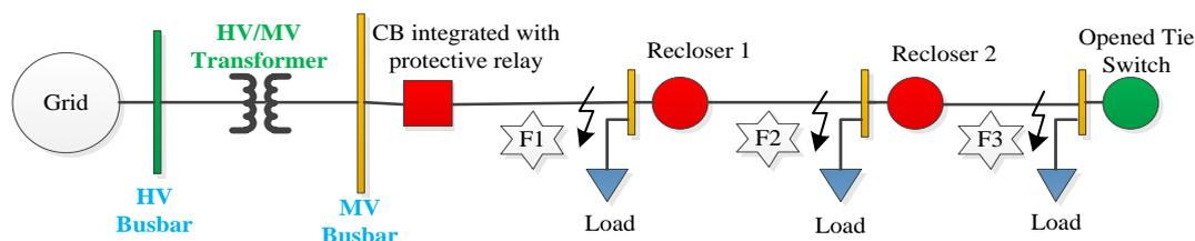
Figure 5. Single-line diagram of a typical feeder of a distribution network.
