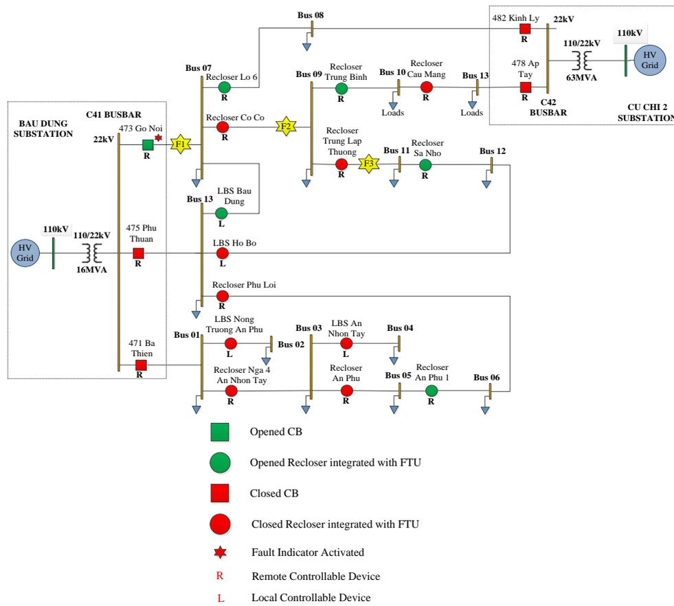
Figure 6. A single-line diagram of 22 kV distribution network with protective devices such as Reclosers, Load Break Switches, and Circuit Breakers and three different fault locations, F1, F2 and F3.
