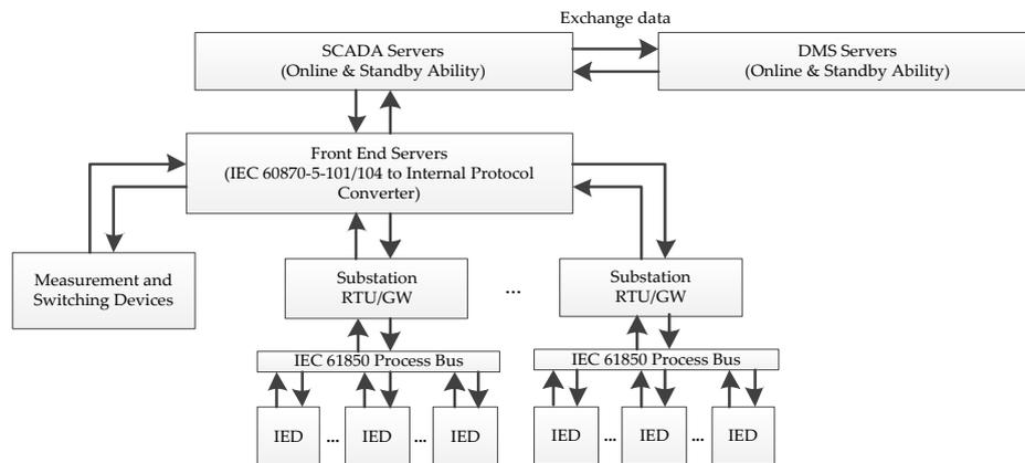
Figure 1. Centralized architecture of DMS for distribution network.
