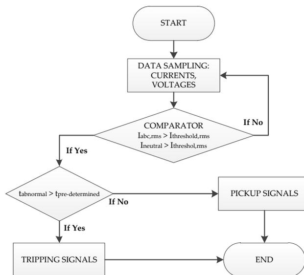
**Figure 4.** Operating principle of overcurrent relays/reclosers ( $I_{abc,rms}$ —phase currents;  $I_{neutral,rms}$ —neutral currents;  $I_{threshold,rms}$ —threshold currents;  $T_{abnormal}$ —the time is counted from fault inception;  $T_{pre-determined}$ —the defined fault detection time; Tripping signal—is given by relays/reclosers; and Pick-up signal—to give a fault alarm from a protective relay.
