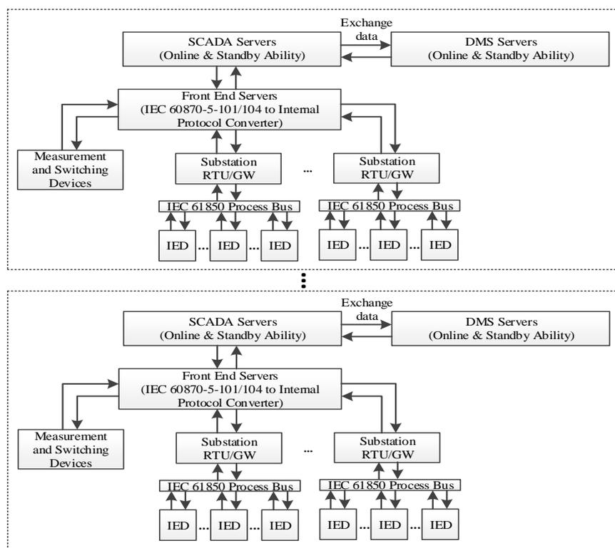
Figure 2. De-centralized architecture of DMS for distribution network.
