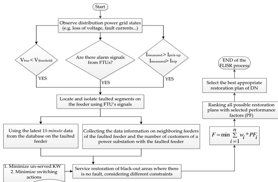
Figure 3. Flow diagram of a proposed FLISR approach for smart distribution networks.
