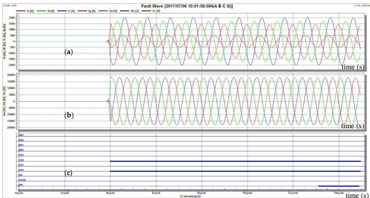
**Figure 10.** Fault waveforms corresponding to a TPGF at F3: (a) three phase currents,  $I_a$  (A),  $I_b$  (A),  $I_c$  (A), and a ground current  $I_g$  (A)); (b) three phase voltages,  $V_a$  (V),  $V_b$  (V), and  $V_c$  (V); (c) tripping signals of the Co-Co recloser (51P2 and 51G2 are respectively phase and ground tripping signals; a TRIP signal shows the tripping action implemented by the recloser).
