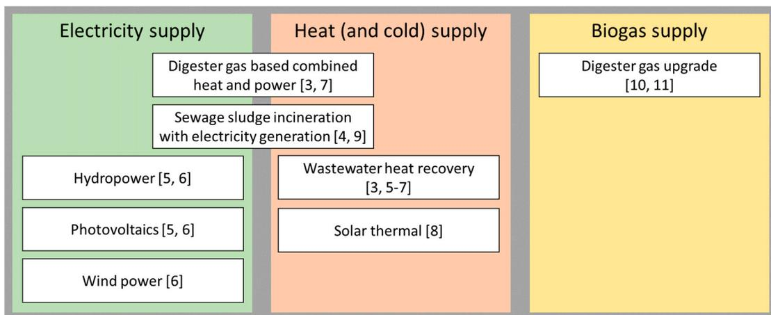
**Figure 1.** Wastewater-based supply of electricity, thermal energy, and biogas [3–11].
