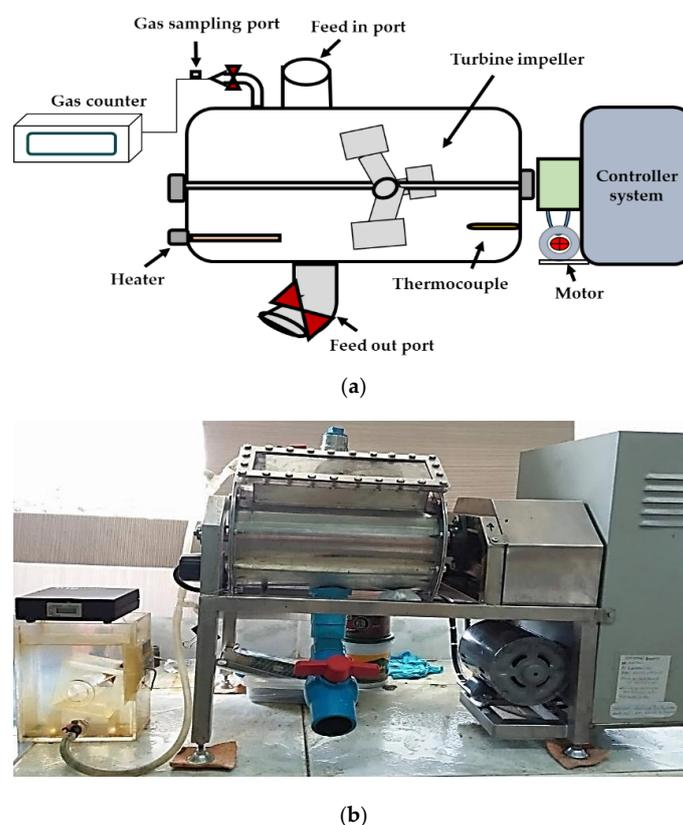
**Figure 3.** Schematic (a) and image (b) horizontal reactor.
