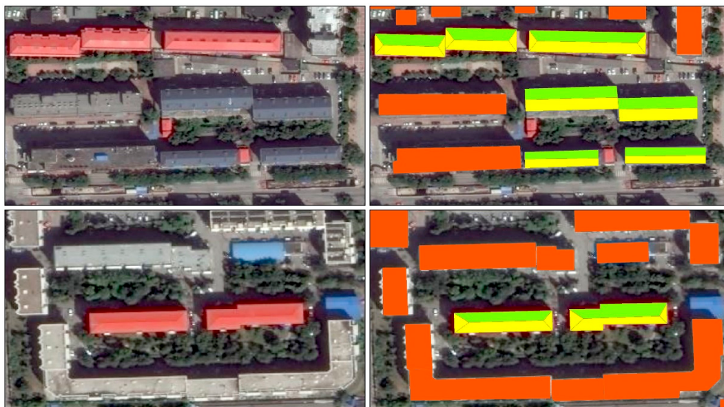
Figure 5. Different types of rooftops (flat rooftops are shown in red and sunny hips and shade hips of pitched roofs are shown in yellow and green, respectively).
