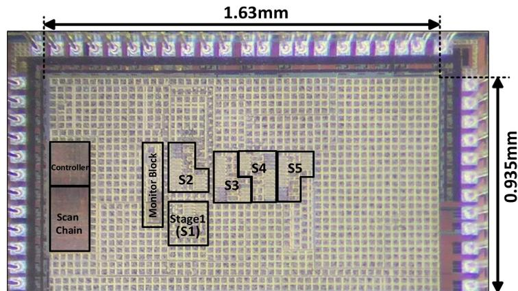
Figure 17. Chip micrograph.
