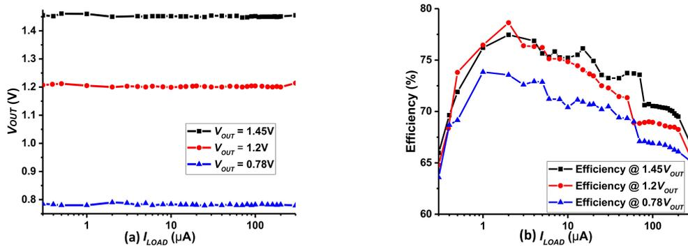
Figure 21. (a) Regulated output voltage vs.  $I_{LOAD}$ . (b) Corresponding efficiencies.
