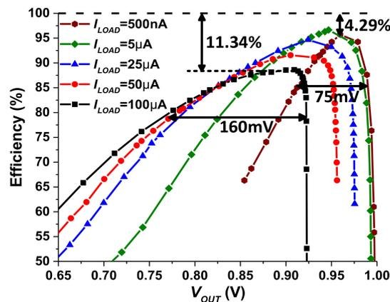
Figure 3. Efficiency of the 2:1 SC converter at varying load.
