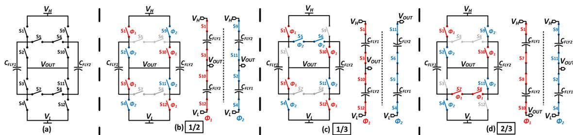
**Figure 8.** Multi-ratio, multi-leaf SC converter stage structure (a) Simplified diagram. (b) Operation scheme for 1/2 ratio. (c) 1/3 ratio. (d) 2/3 ratio.
