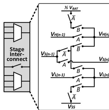
Figure 9. Switch level implementation of the Reconfigurable Stage Interconnection (RSI) scheme.
