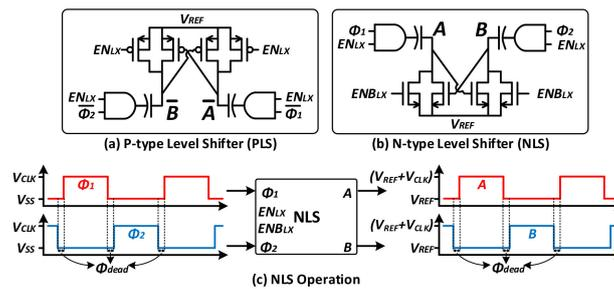
**Figure 13.** Cross coupled level shifter for gate driving (a) P-type level shifter (PLS). (b) N-type level shifter (NLS). (c) N-type level shifter operation.
