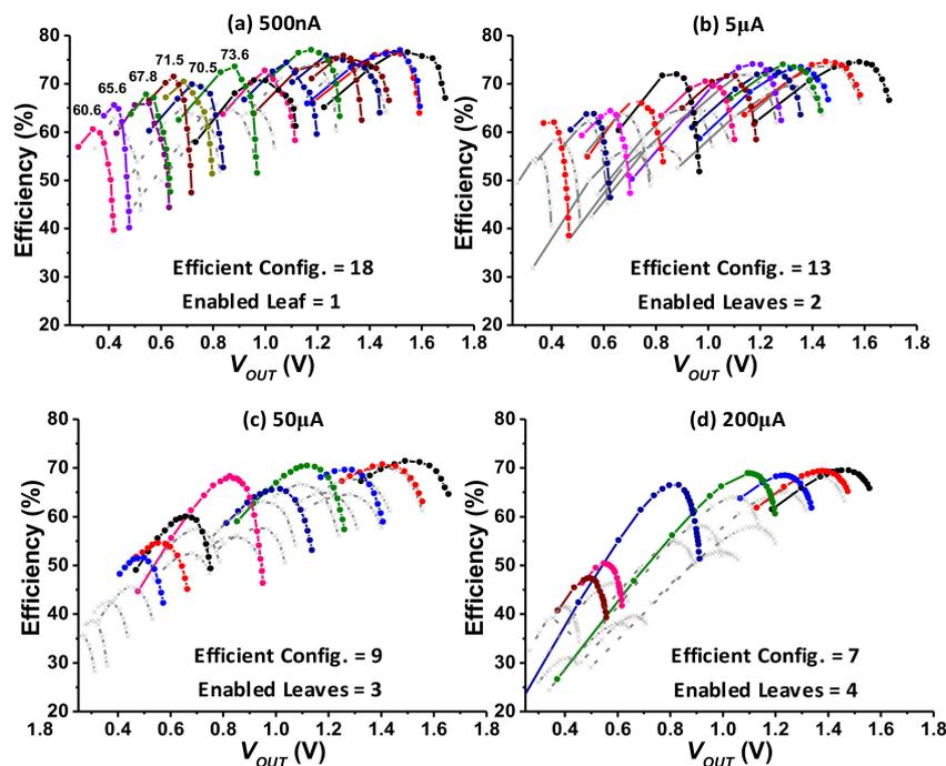
Figure 22. Multi-ratio, multi-leaf SC converter’s efficiency curves at  $I_{LOAD}$  (a) 500 nA. (b) 5  $\mu A$ . (c) 50  $\mu A$ . (d) 200  $\mu A$ .
