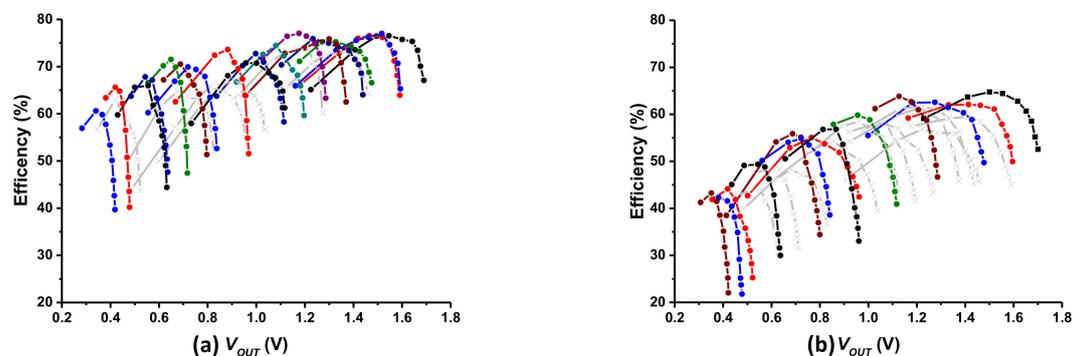
Figure 18. Efficiency vs.  $V_{OUT}$  at  $I_{LOAD} = 500 \text{ nA}$  (a) Only 1 (smallest) leaf enable (Min. switch size). (b) All leaves enabled (Max. switch size).
