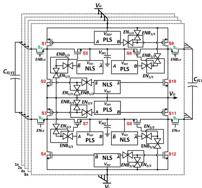
**Figure 7.** Multi-ratio, multi-leaf SC converter stage.
