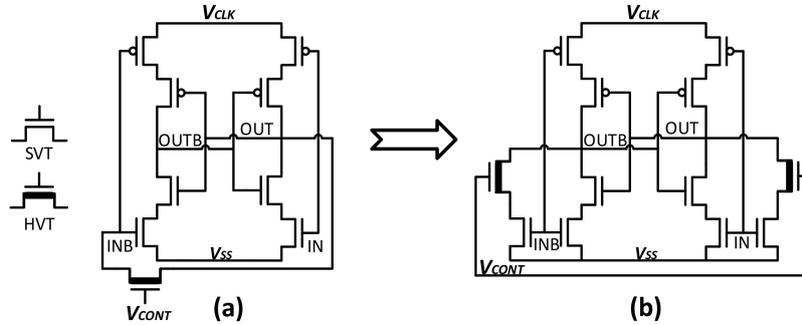
**Figure 14.** Leakage-controlled delay cell (a) Conventional single branch. (b) Modified two leakage control Branches.
