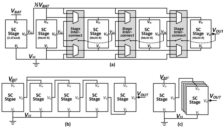
**Figure 6.** Multistage converter (a) Proposed reconfigurable SC topology. (b) Series connected. (c) Parallel connected.
