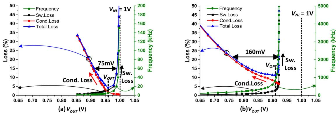
**Figure 2.** Loss contribution in single stage 2:1 SC converter from  $V_{IN} = 2.0$  V (a) Light load (500 nA). (b) Heavy load (100  $\mu$ A).
