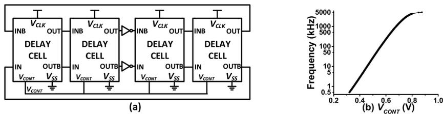
**Figure 15.** (a) Block diagram of leakage-based clock generator. (b) Frequency vs. control voltage ( $V_{CONT}$ ).
