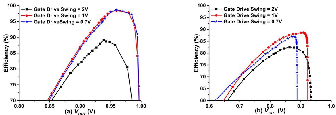
**Figure 5.** Effect of gate drive voltage swing variation  $V_{IN} = 2.0$  V (a) Light load (500 nA). (b) Heavy load (100  $\mu$ A).
