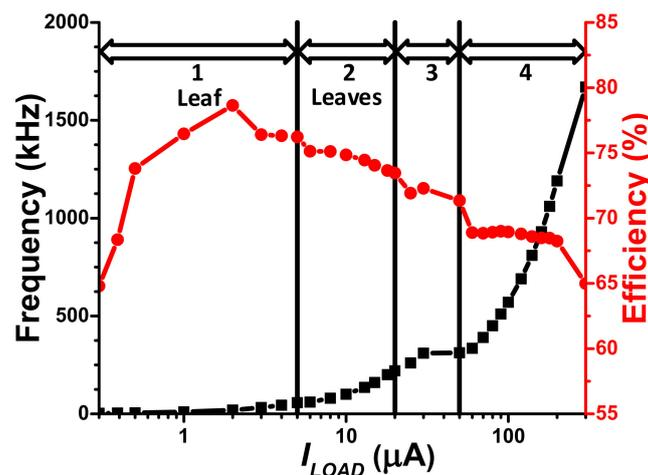
**Figure 20.** Frequency, efficiency and active leaves vs.  $I_{LOAD}$ .
