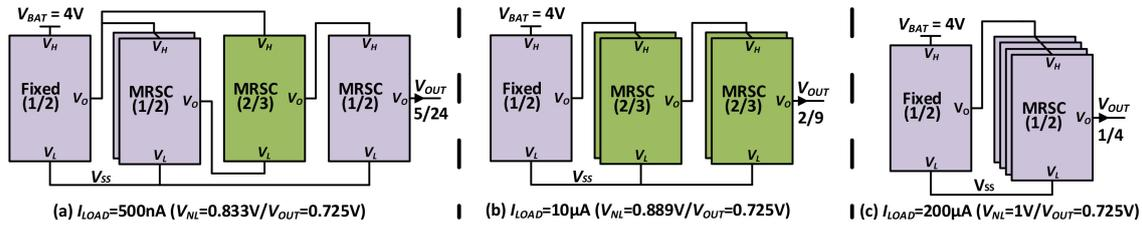
**Figure 12.** Optimal configuration for various load conditions when target  $V_{OUT} = 0.725$  V from  $V_{BAT} = 4.0$  V.
