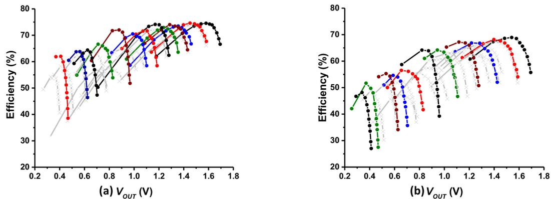
**Figure 19.** Efficiency vs.  $V_{OUT}$  at  $I_{LOAD} = 5 \mu\text{A}$  (a) Leaf 1 and 2 enabled. (b) All leaves enabled (Max. switch size).
