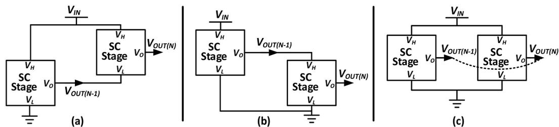
Figure 10. Figure 10. Three possible stage interconnect operation modes: (a)  $A_n B_n = 00$ . (b)  $A_n B_n = 01$ . (c)  $A_n B_n = 1X$ .
