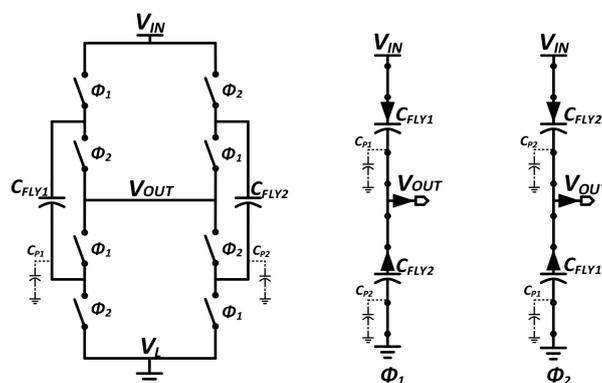
Figure 1. A 2-phase 2:1 step down switched capacitor (SC) converter.
