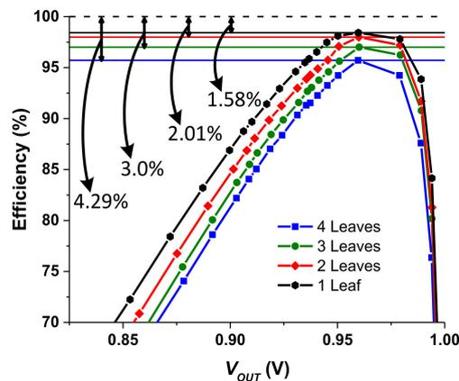
**Figure 4.** Effect of switch width modulation using leaf enable mechanism on efficiency of 2:1 converter at  $I_{LOAD} = 500$  nA.
