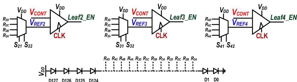
**Figure 16.** Reference comparison circuit for leaf control with  $V_{CONT}$ .
