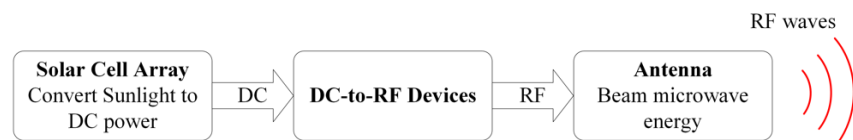
Figure 2. Basic structure schematic diagram of wireless power transmission (WPT) via microwave radiation.
