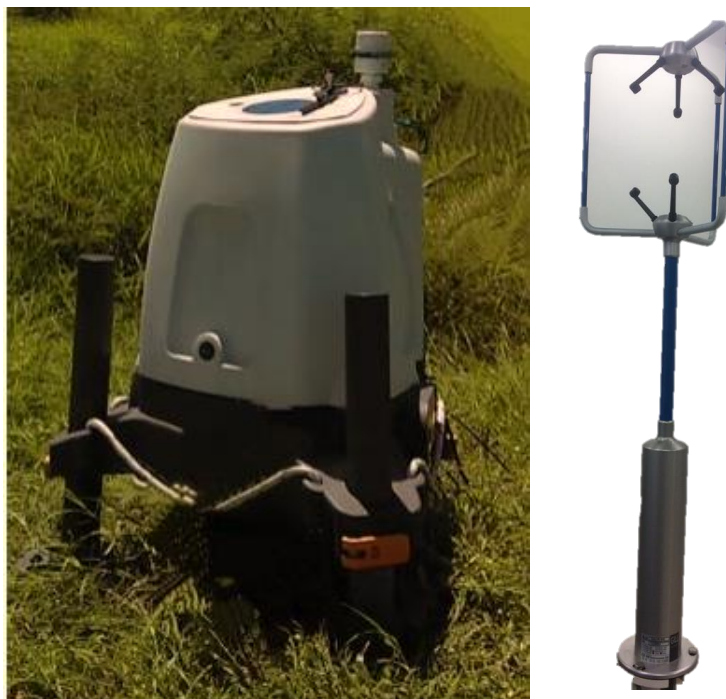
Figure 3. ZephIR LIDAR 300 (left) and 3D Gill WindMaster ultrasonic anemometer (right).
