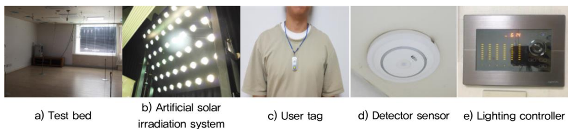
Figure 3. Overview of test bed and measurement apparatus.
