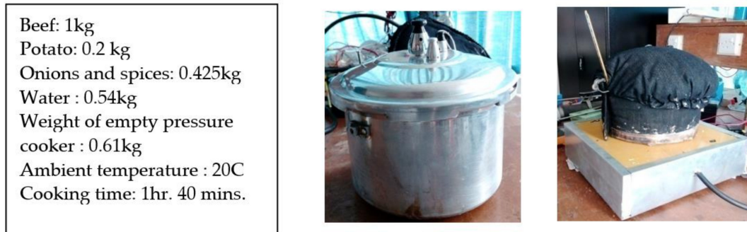
Figure 5. Experimental setup for e-cooking using pressure cooker.
