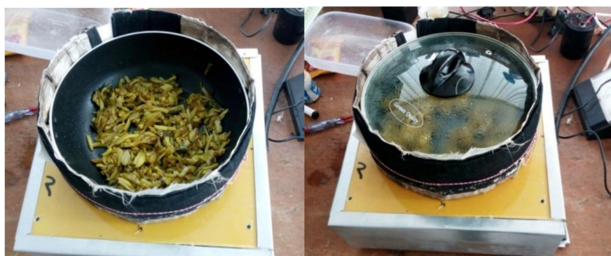
Figure 6. Arrangement for the potato chip frying in the e-cooker.
