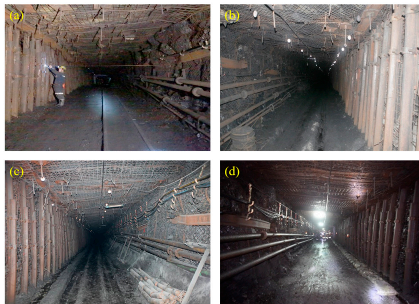
Figure 19. Effects of the surrounding rock control in the Dianping coal mine. (a) 100 m from open-off cut; (b) 200 m from open-off cut; (c) 300 m from open-off cut; (d) 400 m from open-off cut.
