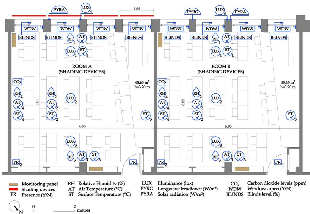
Figure 2. Floor plan showing the location of the sensors in the classrooms monitored.
