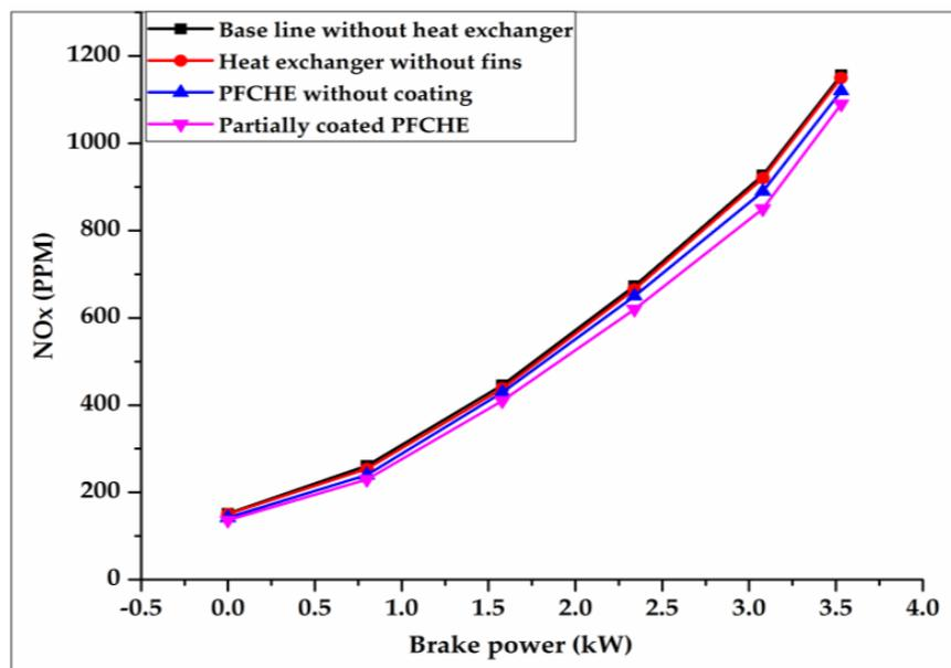
Figure 11. Effect of heat exchanger on NO<sub>x</sub> emission.
