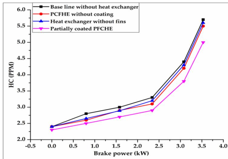
Figure 9. Effect of heat exchanger on HC emission.
