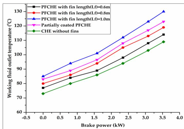
Figure 5. Variation of working fluid outlet temperature with fin geometry.
