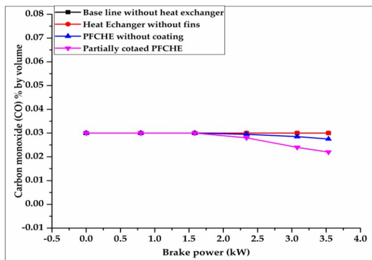
Figure 10. Effect of heat exchanger on CO emission.
