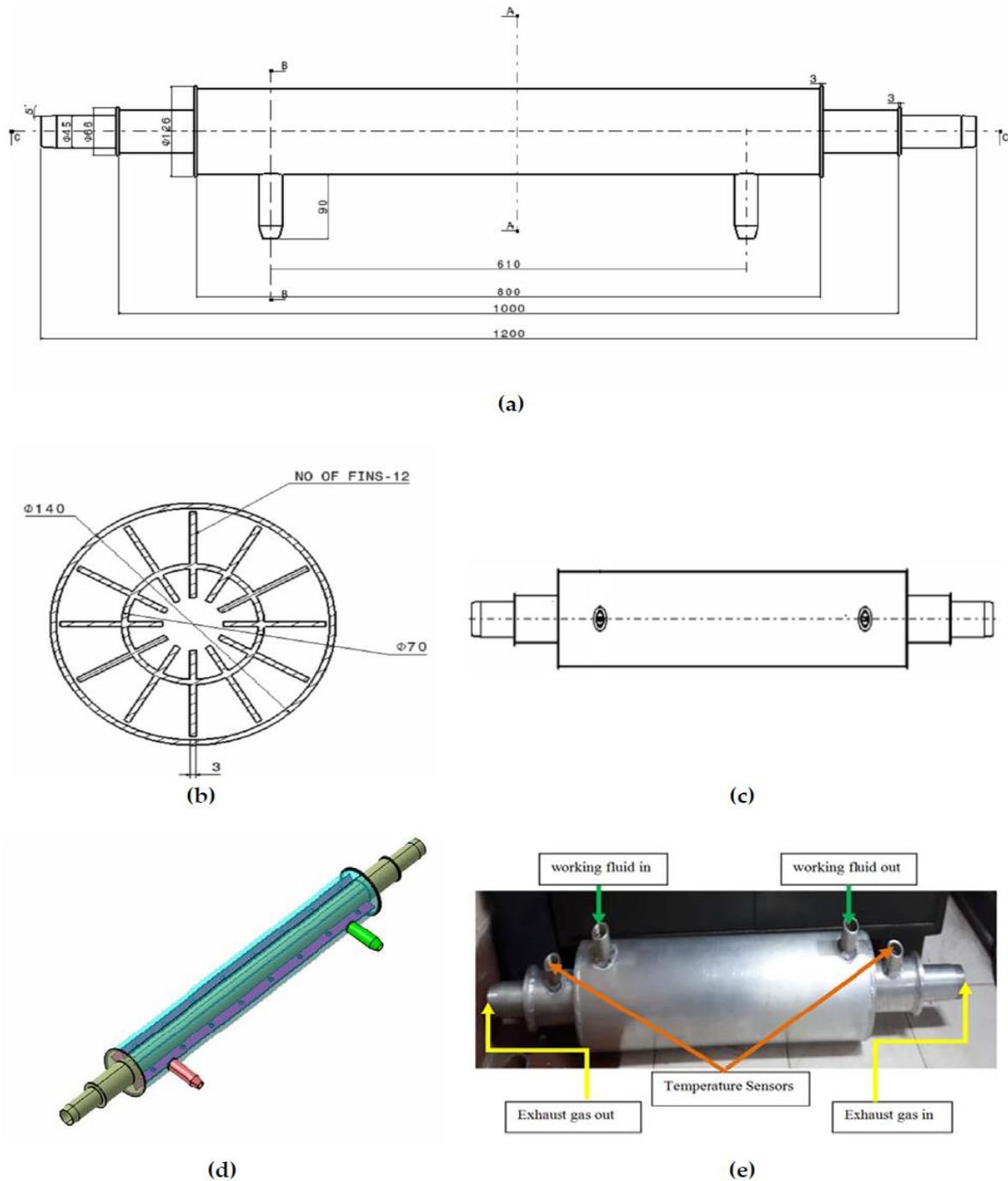
**Figure 3.** Schematic sketch of 2-Dimensional, 3-Dimensional and fabricated heat exchanger views of PFCHE. (a) Front view, (b) Side view, (c) Top view, (d) Isometric view, (e) Fabricated view.
