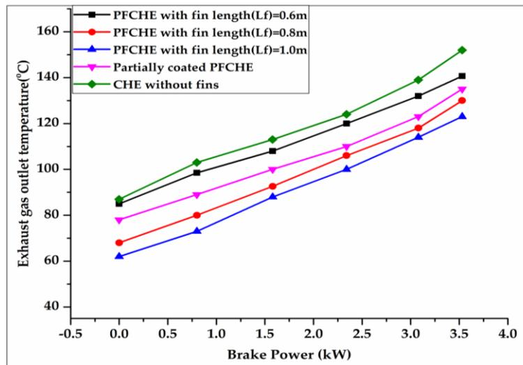
Figure 4. Variation of exhaust gas outlet temperature with fin geometry.
