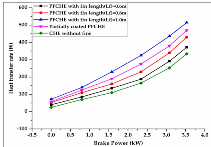
Figure 6. Variation of heat transfer rate with fin geometry.
