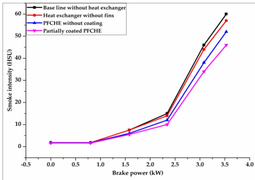
Figure 13. Effect of heat exchanger on smoke intensity.
