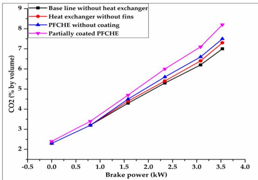
Figure 12. Effect of heat exchanger on CO<sub>2</sub> emission.
