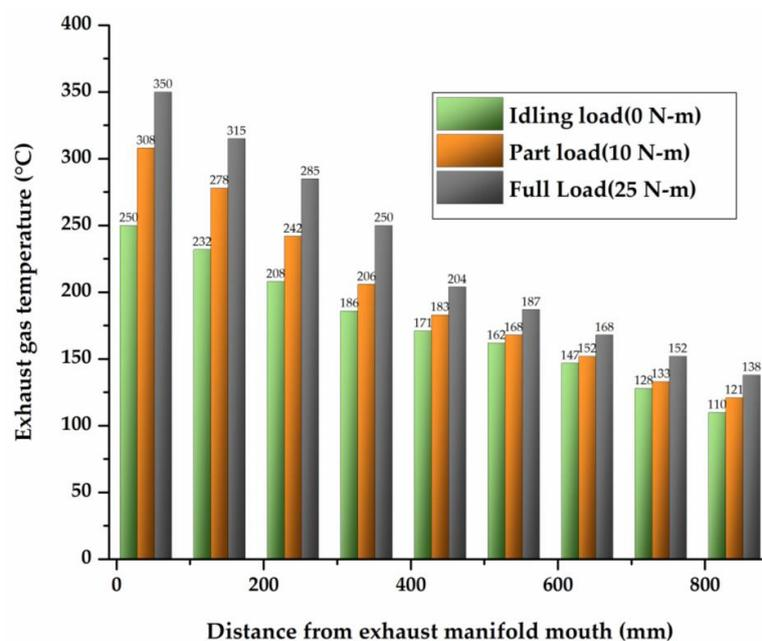
Figure 2. Exhaust gases temperature at different locations.
