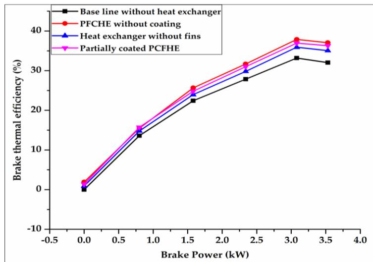
Figure 8. Effect of waste heat recovery (WHR) on brake thermal efficiency.
