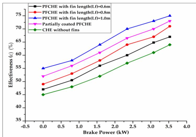
Figure 7. Effectiveness of heat exchanger with fin geometry.
