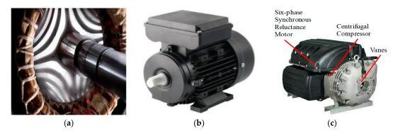
**Figure 12.** Completed photo pictures of six-phase synchronous reluctance motor: (**a**) stator, rotor and winding; (**b**) combination; (**c**) six-phase synchronous reluctance motor mounted to a centrifugal compressor.
