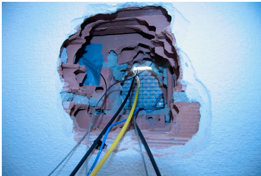
Figure 11. The location of sensors N_1 to N_5 in the enclosure layers.
