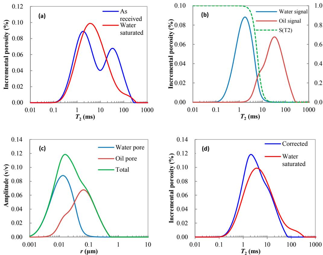
**Figure 7.** Sample M1: (a)  $T_2$  distributions for “as received” state and water saturated state; (b) Water and oil signal distributions obtained from “as received” state  $T_2$  distribution using weight function  $S(T_2)$ ; (c) Water-containing pore, oil-bearing pore and total pore size distributions; (d) Comparison of corrected and measured  $T_2$  distributions for water-saturated state.
