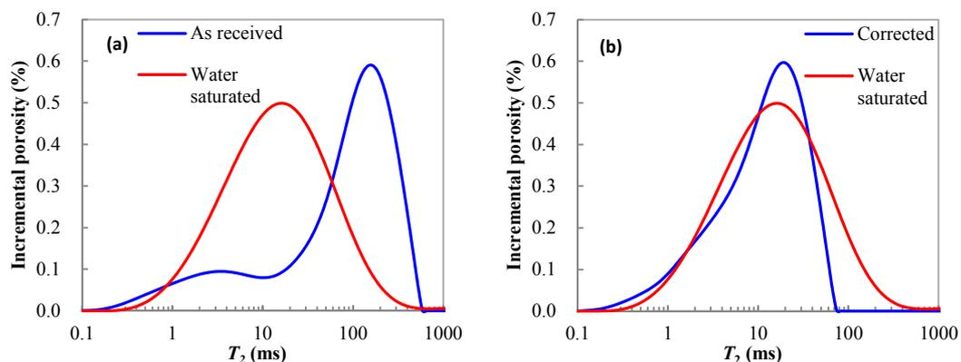
**Figure 8.** Sample M2: (a)  $T_2$  distributions for “as received” state and water saturated state; (b) Comparison of corrected and measured  $T_2$  distributions for water-saturated state.
