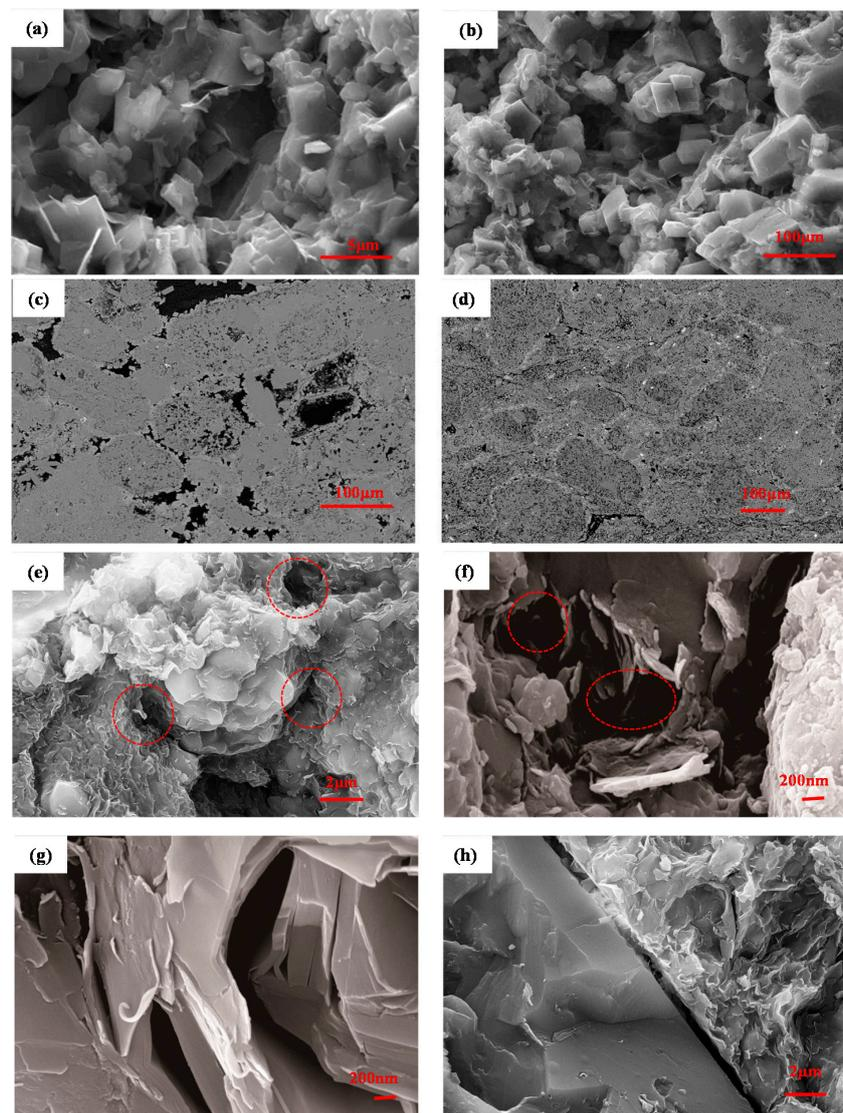
**Figure 2.** The pore types according to SEM analysis. (a) Intergranular dissolved pores; (b) Intergranular dissolved pores; (c) Intergranular and intragranular dissolved pores; (d) Intergranular and intragranular dissolved pores; (e) Illite/smectite mixed layer clay pores; (f) Chlorite clay pores; (g) Fracture pore; (h) Fracture pore.
