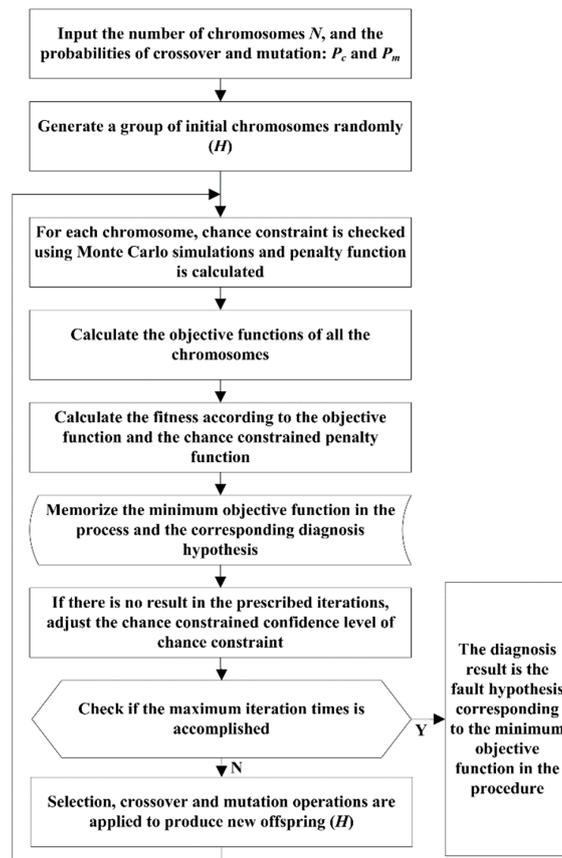
Figure 3. The flowchart of the solving procedure.
