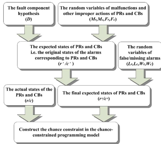
Figure 2. The flowchart of the establishment of the chance constraint.
