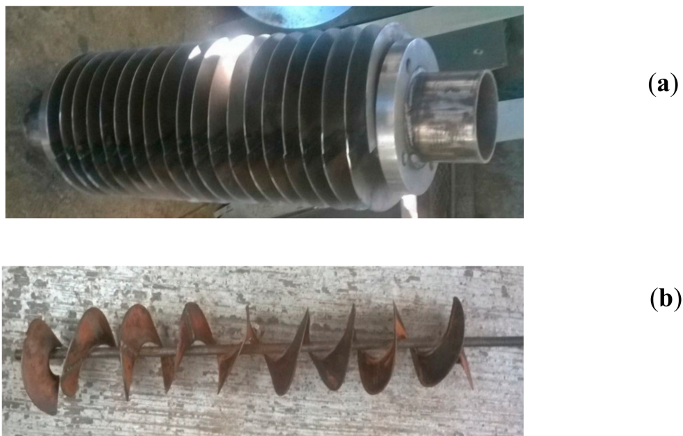
Figure 3. Picture of the helical mixer inserted in the (a) annulus and (b) central tube.
