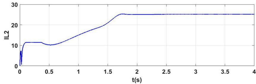
**Figure 10.** Inverter output current  $I_{L2}$ , affected by optimal levels for micro-grid and network parameters.
