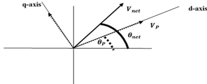
Figure 6. Diagram of network voltage and measured voltage by PLL.
