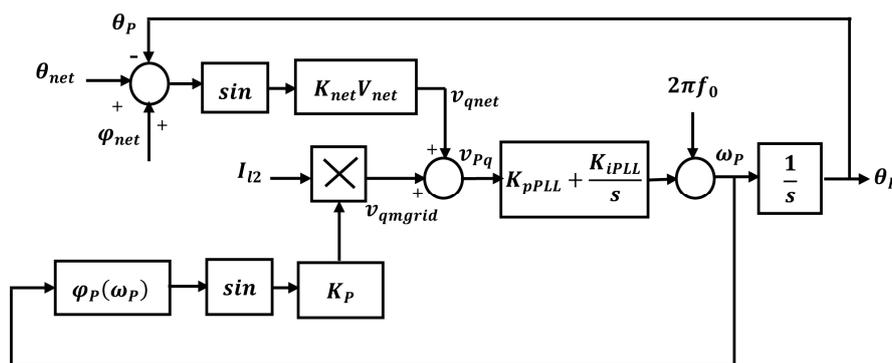
Figure 7. Block diagram of PLL, affected by network and micro-grid side factors.
