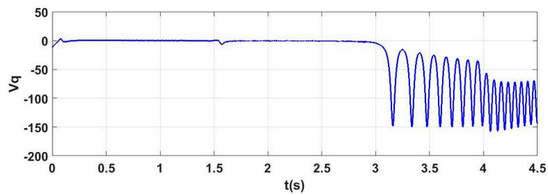
Figure 19. Voltage  $v_q$  measured by PLL for  $C_{sc} = 0.1$  F.
