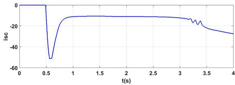
Figure 18. Super-capacitor current, affected by optimal levels for  $C_{sc} = 0.1$  F.
