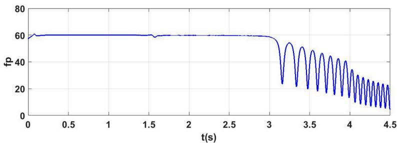
Figure 20. Output frequency of PLL for  $C_{sc} = 0.1$  F.
