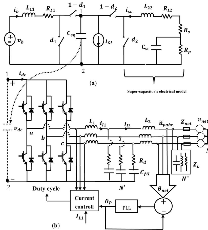
**Figure 1.** Schematic of studied micro-grid: (a) the hybrid storage system and equivalent circuit of micro-grid (b) network-interface converter and local load.
