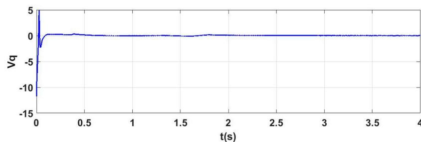
**Figure 9.** Voltage  $v_q$  measured by PLL, affected by optimal levels for micro-grid and network parameters.
