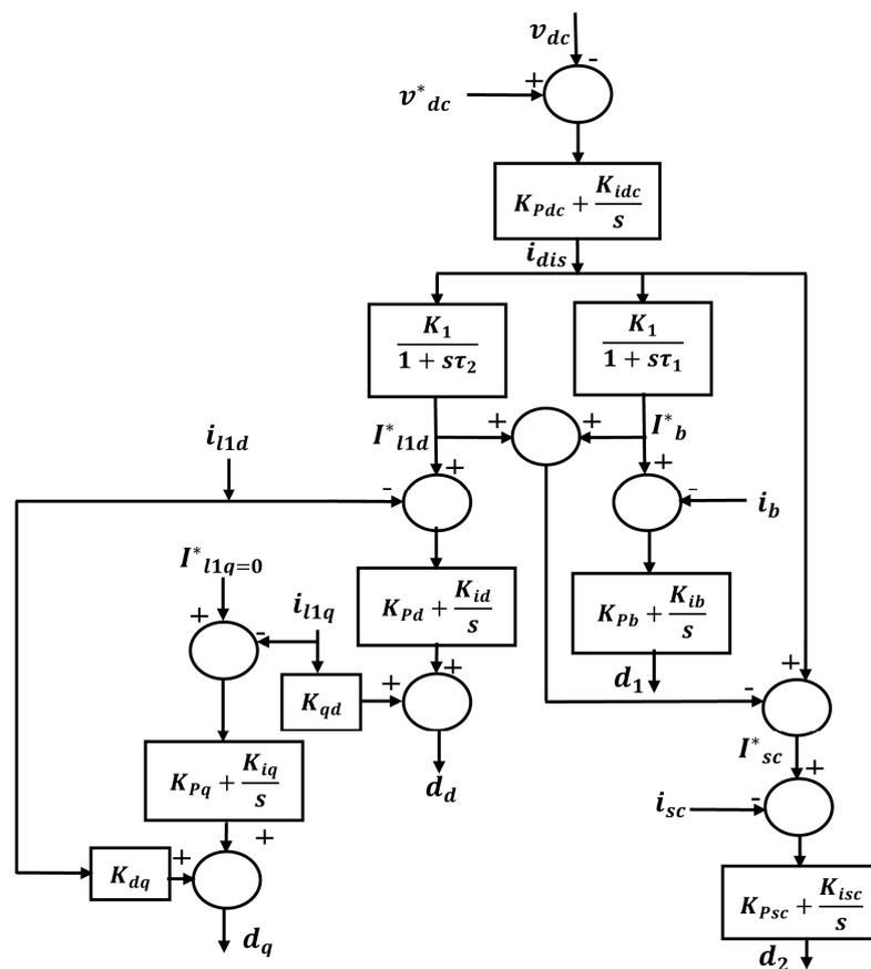
Figure 2. Proposed control system for hybrid storage system and network-interface converter.
