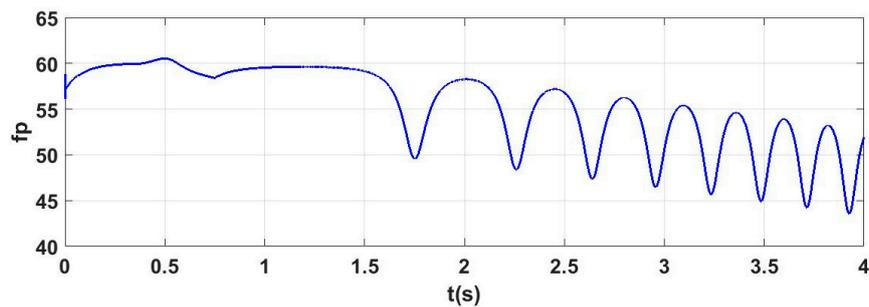
Figure 16. Output frequency of PLL for  $\tau = 0.5$  s.
