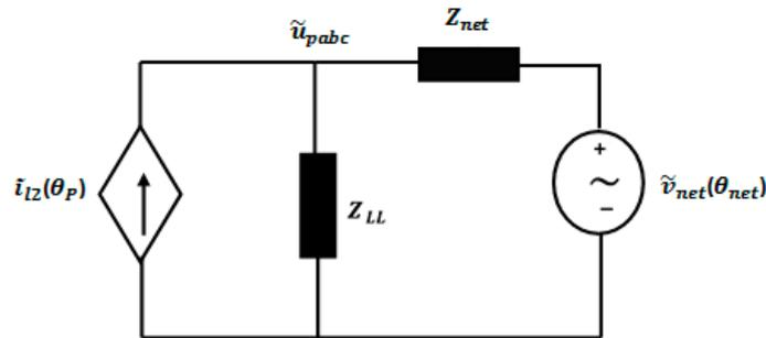
**Figure 5.** Simplified equivalent circuit of studied micro-grid and grid-side converter.
