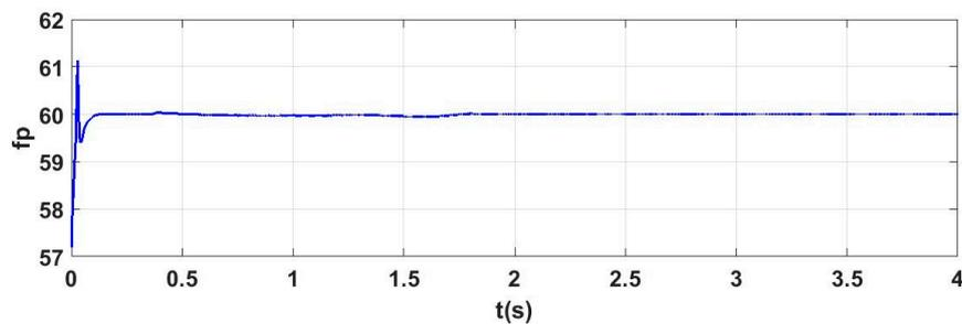
**Figure 11.** Output frequency of PLL, affected by optimal levels for micro-grid and network parameters.
