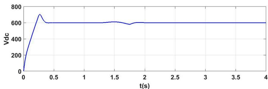
**Figure 12.** DC bus voltage, affected by optimal levels for micro-grid and network parameters.
