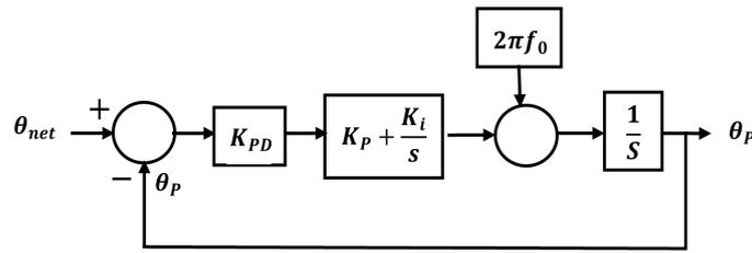
Figure 3. Linear model of SRF-PLL [12].
