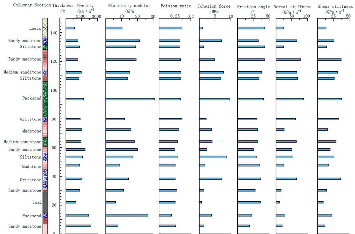
Figure 2. Composite column and mechanical parameters of working face 1313.
