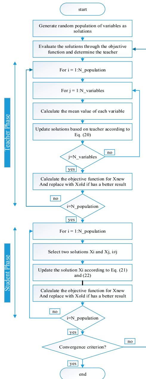
Figure 2. Flowchart of the TLBO algorithm.
