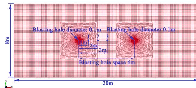
Figure 10. DHB numerical simulation model.
