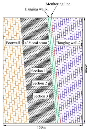
Figure 5. HSTCC numerical simulation model.
