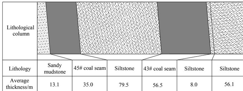
Figure 3. Stratigraphic column of the 4301 working face.
