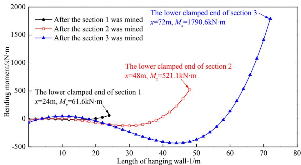
Figure 9. Bending moment distribution of the hanging wall-1.
