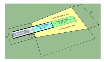
**Figure 2.** Surface areas with and near the end of a runway [39], which cannot be used for PV deployment. Only surface areas coated in green can be used for PV.
