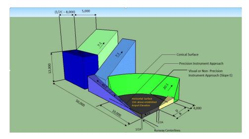
**Figure 1.** Defining aerial zones defined for airports, which are adapted from [60]. The lower right is the region of relevance for photovoltaics (PV) systems. The primary surface is a surface longitudinally centered on a runway shown in blue, a horizontal plane 150 ft. above the established airport elevation is shown in dark grey, and the conical surface is shown in green.
