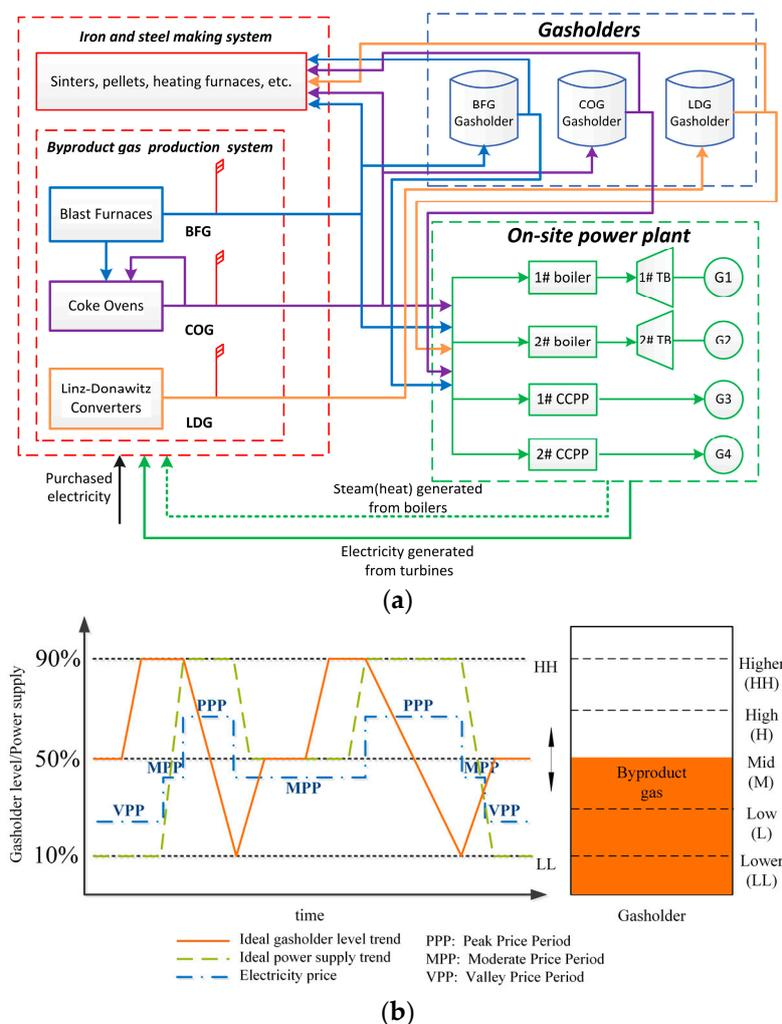
**Figure 1.** (a) Diagram of a byproduct gas system in a steel plant; (b) schematic view of the collaboration between the gasholder level and the electricity generation of the on-site power plant (OSPP) under the time-of-use (TOU) tariff.
