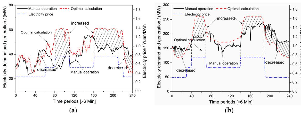
**Figure 2.** (a) Electricity generation of plant A in each period before and after optimization; (b) electricity generation of plant B in each period before and after optimization.
