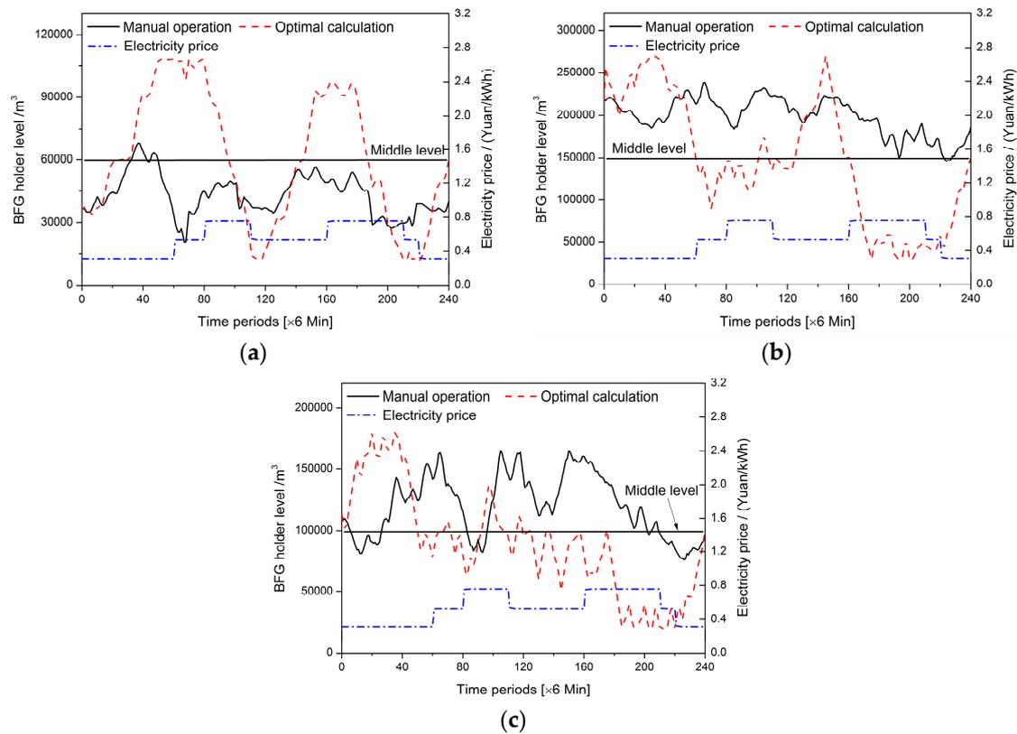
**Figure 3.** (a) Comparison of manual operation and optimal calculation results for the 120,000 m<sup>3</sup> (Blast furnace gas) BFG holder of plant A; (b) comparison of manual operation and optimal calculation results for the 300,000 m<sup>3</sup> (Blast furnace gas) BFG holder of plant B; (c) comparison of manual operation and optimal calculation results for the 200,000 m<sup>3</sup> (Blast furnace gas) BFG holder of plant B.
