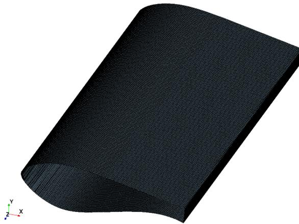
Figure 4. The surface mesh on the airfoil.
