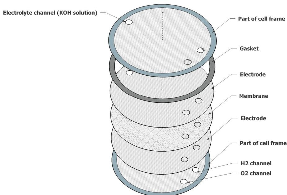
**Figure 1.** Alkaline electrolysis cell set-up (based on [22]).
