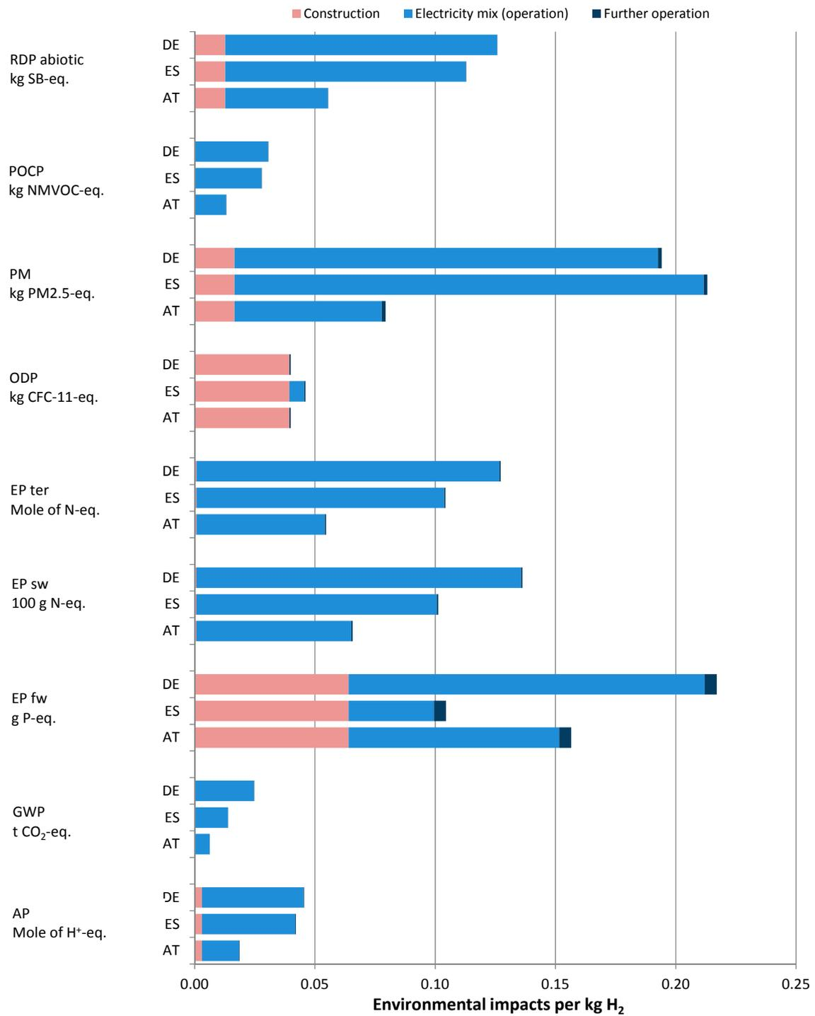
Figure 3. Share of life cycle stages on the impact categories at different sites of operation.
