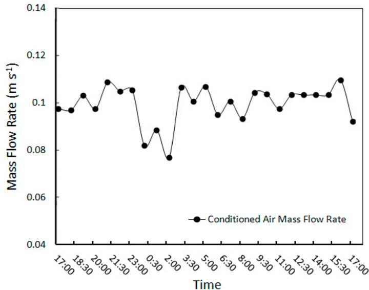
**Figure 18.** The conditioned air mass flow rate from the wind tower outlet to the room for test No. 5 (from 5:15 p.m. on the 22nd to 5:15 p.m. on the 23rd of August 2013).
