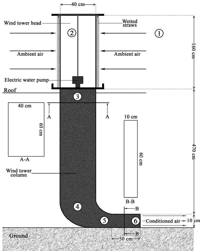
**Figure 8.** Cross-sectional view of the modular wind tower with wetted surfaces. Numbers in circles (1 to 6) have been used as subscripts hereinafter.
