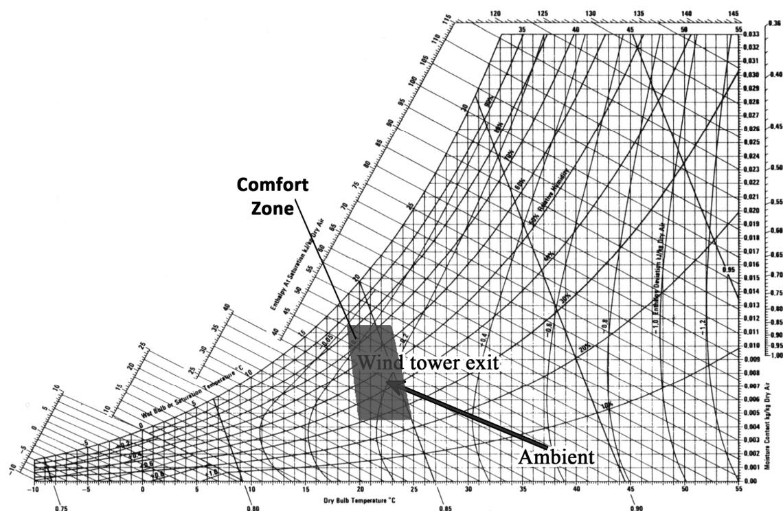
**Figure 19.** Property changes of the air passing throughout the modular wind tower with wetted surfaces.
