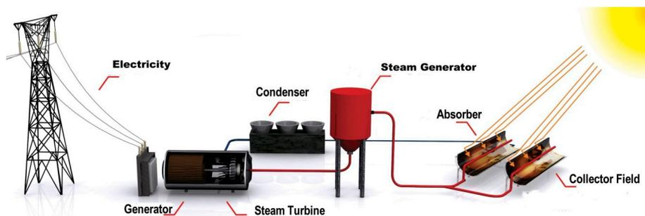
**Figure 2.** Scheme of solar thermal power plant.
