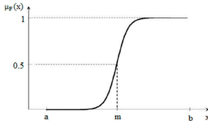
**Figure 10.** Fuzzy sigmoidal membership function.  $U$  is a given set Universe. A fuzzy subset  $F$  from  $U$  is characterized by a membership function, represented by  $\mu_F: U \rightarrow [0,1]$ , which associates to each  $x \in U$ , a real number  $\mu_F(x)$  defined in the interval  $[0,1]$ . This representation allows a gradual transition between the membership ( $\mu_F(x) = 1$ ) and the non-membership ( $\mu_F(x) = 0$ ) [28].
