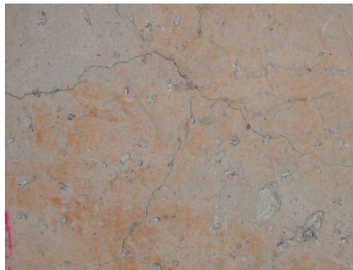
Figure 1. Pre-existing fractures on the surface of a block after heat and cooling treatments from Zhou et al. [16].
