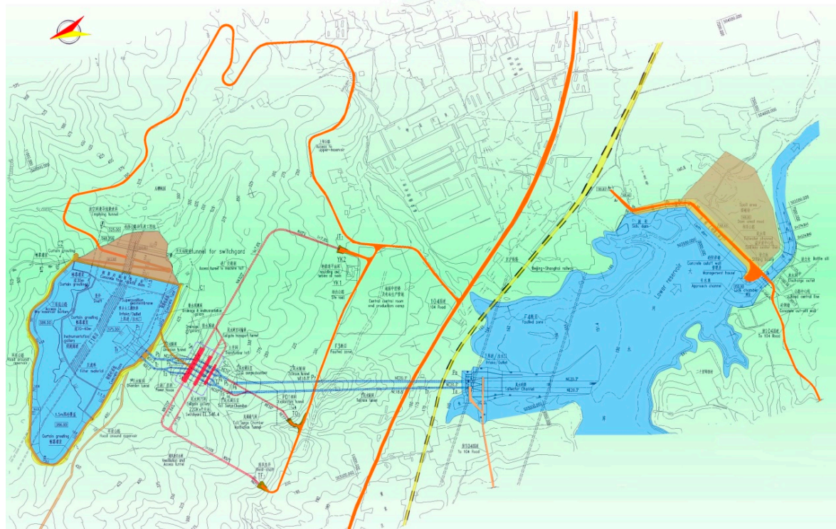
Figure 4. Layout diagram of the Taishan pumped-storage hydropower station.
