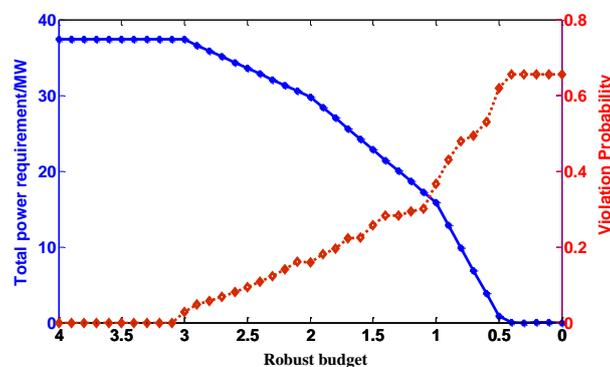
**Figure 4.** Power capacity of energy storage and the corresponding violation probability versus the robust budget.
