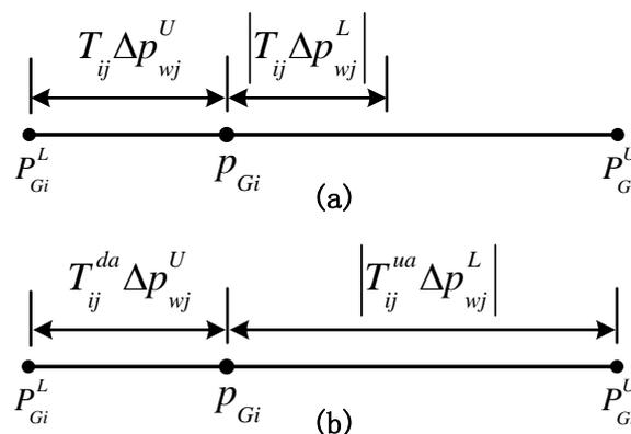
**Figure 1.** (a) Employing the same variable  $T_{ij}$  to model the upward and downward adjustment from  $i$ th generator; (b) Employing different variables,  $T_{ij}^{ua}$  and  $T_{ij}^{da}$ , to optimize the upward and downward adjustment of  $i$ th dispatchable generator.
