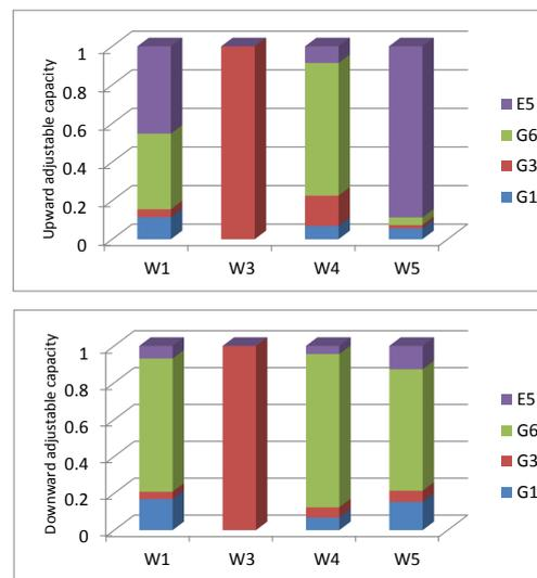
**Figure 3.** Upward and downward adjustable coefficients of dispatchable generators and energy storage to accommodate wind power.
