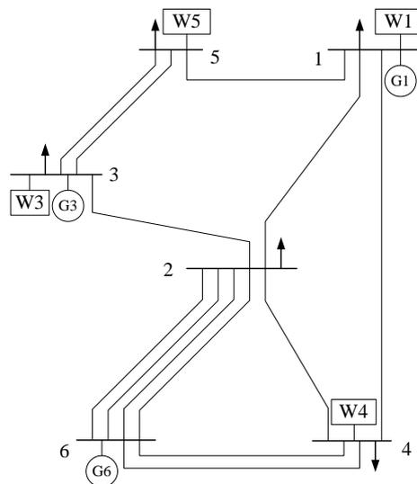
**Figure 2.** Topology of modified Garver 6-bus system.
