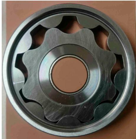
**Figure 6.** GeroMAG trochoidal gear set.
