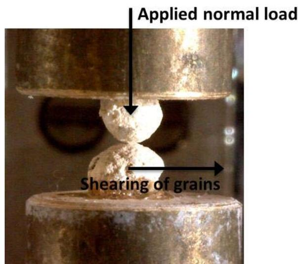
**Figure 6.** Image of CDV granules in contact during the setup of a micromechanical sliding experiment.
