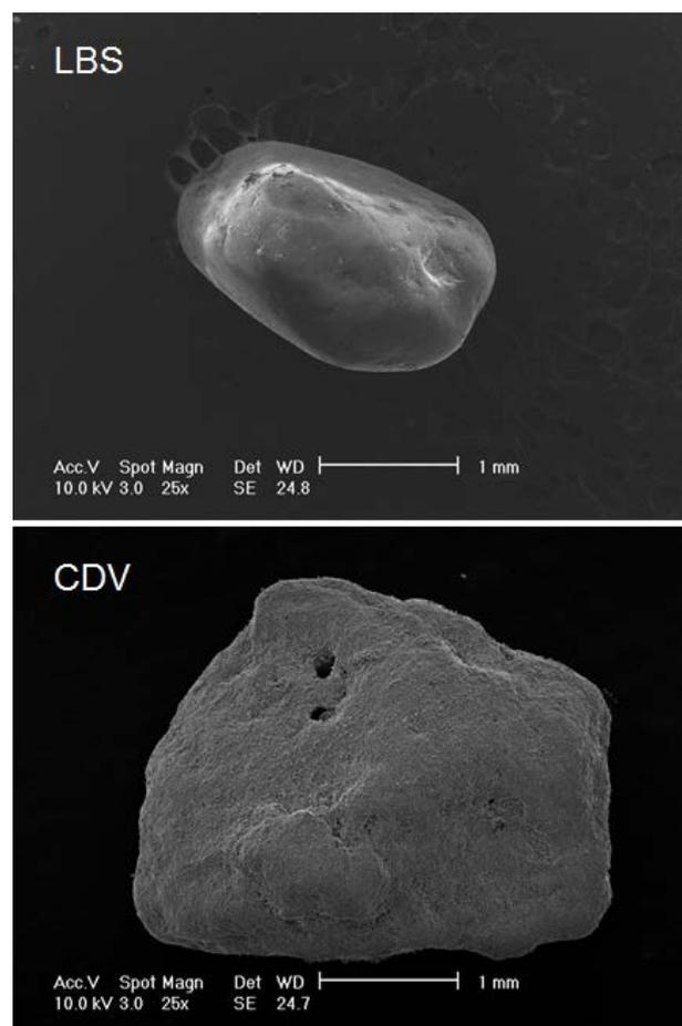
**Figure 1.** Scanning electron microscope images of LBS grain (**top**) and CDV granule (**bottom**) indicating their outline.
