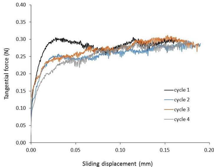
**Figure 18.** Tangential force–displacement plot at the contacts of CDV granules indicating the effect of the shearing cycle (tests at a normal load of 0.5 N).
