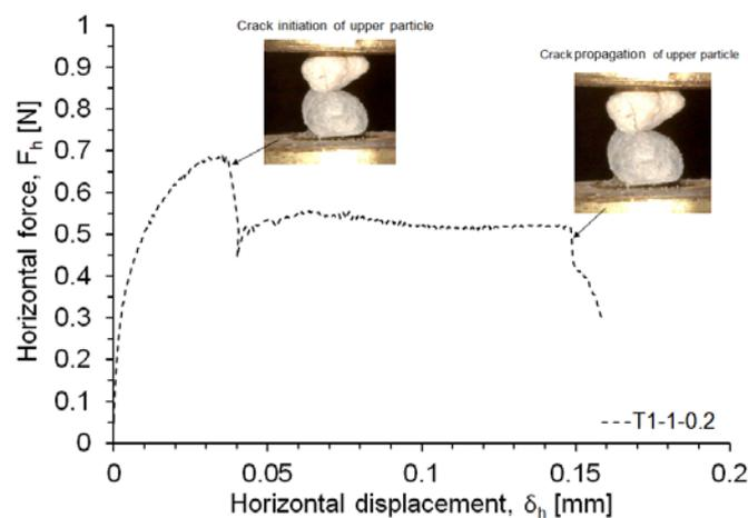
**Figure 10.** Sliding experiment on CDV granules with observation of crack initiation and propagation during shearing.
