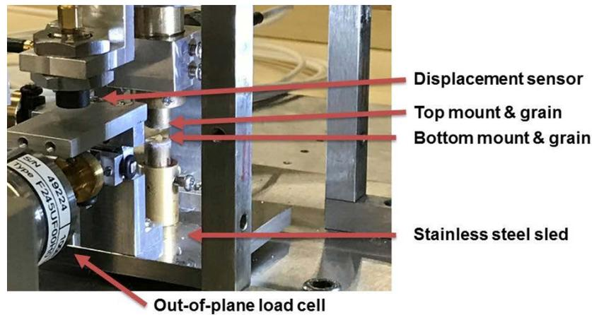
**Figure 5.** Close-up view of the micromechanical sliding apparatus of City University of Hong Kong during the set of a test on LBS grains.
