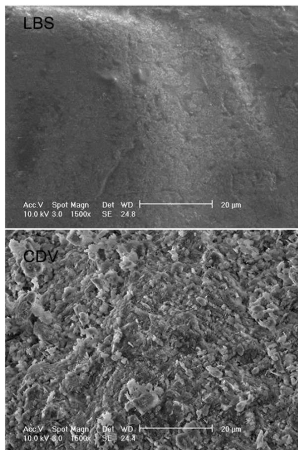
**Figure 2.** Close image from scanning electron microscope of LBS grain (**top**) and CDV granule (**bottom**) indicating their surface characteristics.
