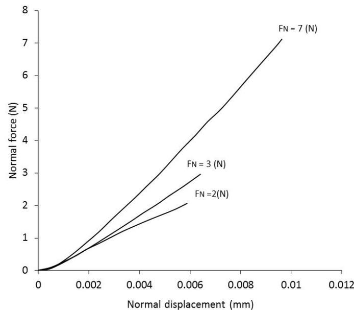
**Figure 11.** Typical plots of normal force–displacement at the contacts of LBS grains.
