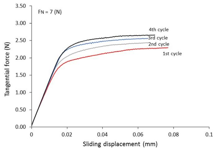
**Figure 15.** Tangential force–displacement plots at the contacts of LBS grains indicating the effect of the shearing cycle at a normal force of 7 N.
