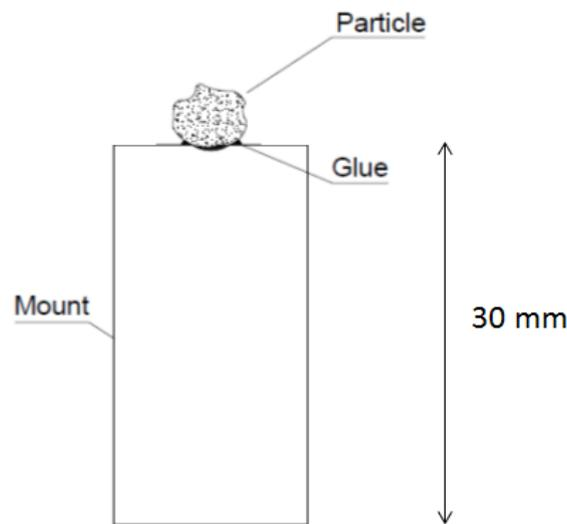
**Figure 9.** Schematic illustration of grain–brass mount system (after Senetakis et al. [6] with modifications by the authors).
