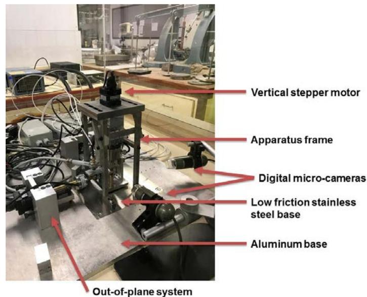
**Figure 3.** Image of the micromechanical sliding apparatus of City University of Hong Kong.
