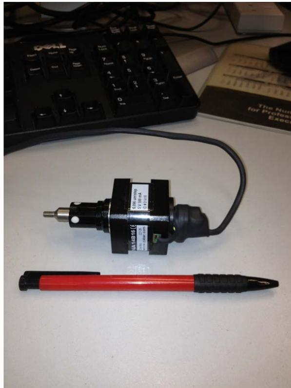
**Figure 7.** Image of a linear micro-stepper motor which is part of the micromechanical sliding apparatus.
