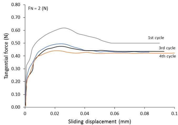
**Figure 14.** Tangential force–displacement plots at the contacts of LBS grains indicating the effect of the shearing cycle at a normal force of 2 N.
