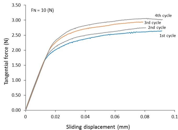
**Figure 16.** Tangential force–displacement plots at the contacts of LBS grains indicating the effect of the shearing cycle at a normal force of 10 N.
