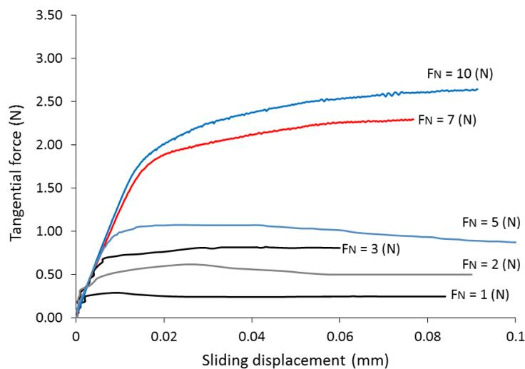
**Figure 12.** Tangential force–displacement plot at the contacts of LBS grains and the effect of the applied normal load (tests during the first shearing cycle).
