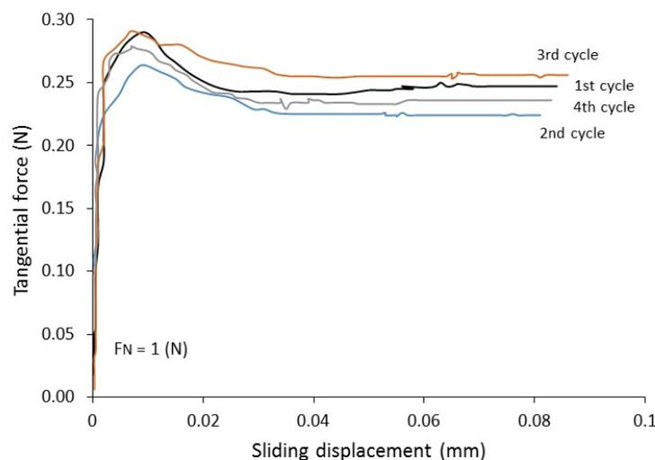
**Figure 13.** Tangential force–displacement plots at the contacts of LBS grains indicating the effect of the shearing cycle at a normal force of 1 N.
