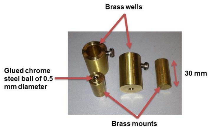
**Figure 8.** Image of brass mounts and wells used to mount the grains for the micromechanical sliding tests.
