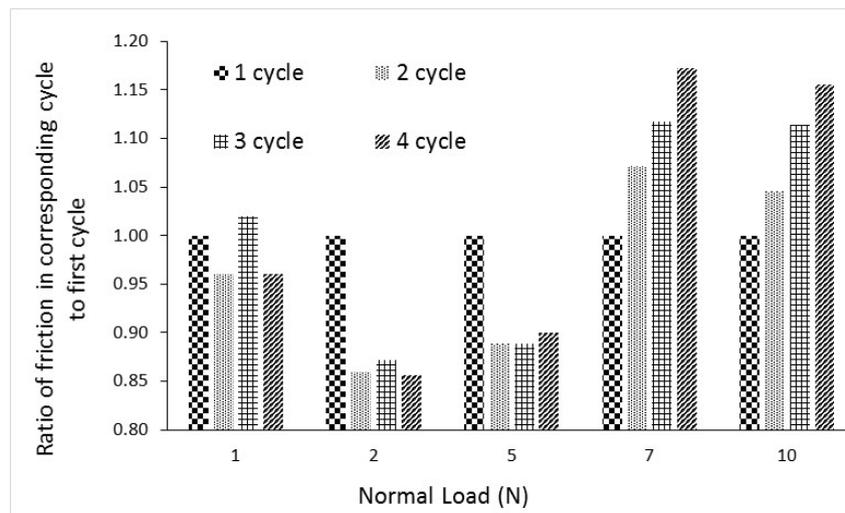
**Figure 17.** The effect of the shearing cycles on the inter-particle friction ratio of LBS grains.
