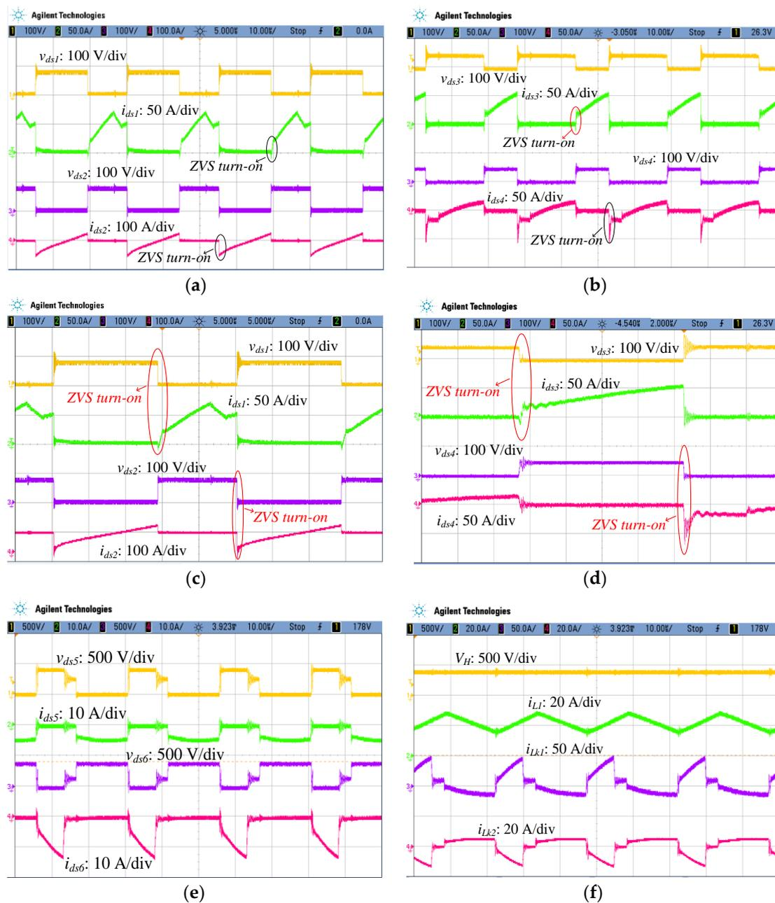
**Figure 13.** Experimental results in step-up mode operation at  $P_o = 1$  kW: (a) measurements from  $S_1$  and  $S_2$ ; (b) measurements from  $S_3$  and  $S_4$ ; (c) zoomed-in waveforms measured from  $S_1$  and  $S_2$ ; (d) zoomed-in waveforms of  $S_3$  and  $S_4$ ; (e) measurements from  $S_5$  and  $S_6$ ; and (f) waveforms of  $V_H$ ,  $i_{L1}$ ,  $i_{Lk1}$ , and  $i_{Lk2}$ .
