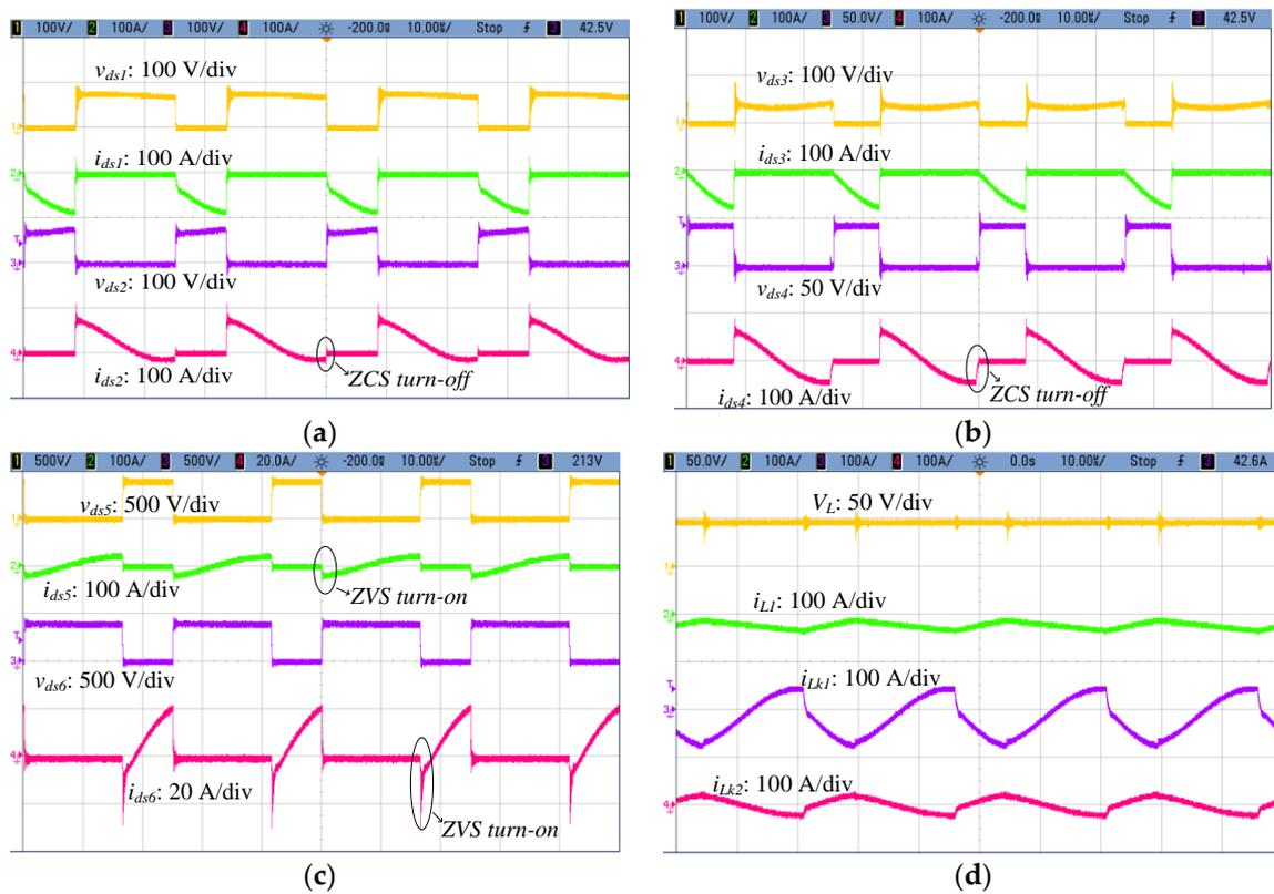
**Figure 14.** Experimental results in step-down mode operation at  $P_o = 1$  kW: (a) measurements from  $S_1$  and  $S_2$ ; (b)  $S_3$  and  $S_4$ ; and (c)  $S_5$  and  $S_6$ ; and (d) the waveforms of  $V_L$ ,  $i_{L1}$ ,  $i_{Lk1}$ , and  $i_{Lk2}$ .
