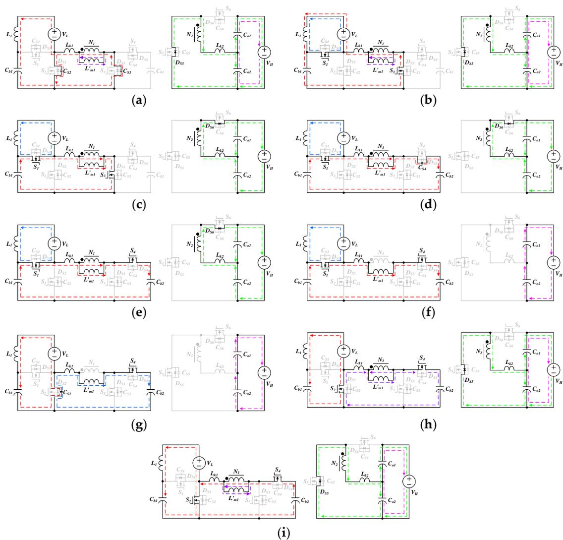
**Figure 3.** Equivalent circuit of proposed bidirectional converter in step-up mode: (a) Stage 1; (b) Stage 2; (c) Stage 3; (d) Stage 4; (e) Stage 5; (f) Stage 6; (g) Stage 7; (h) Stage 8; and (i) Stage 9.
