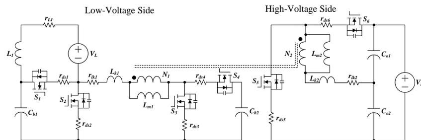
Figure 10. The non-ideal equivalent circuit of the converter.
