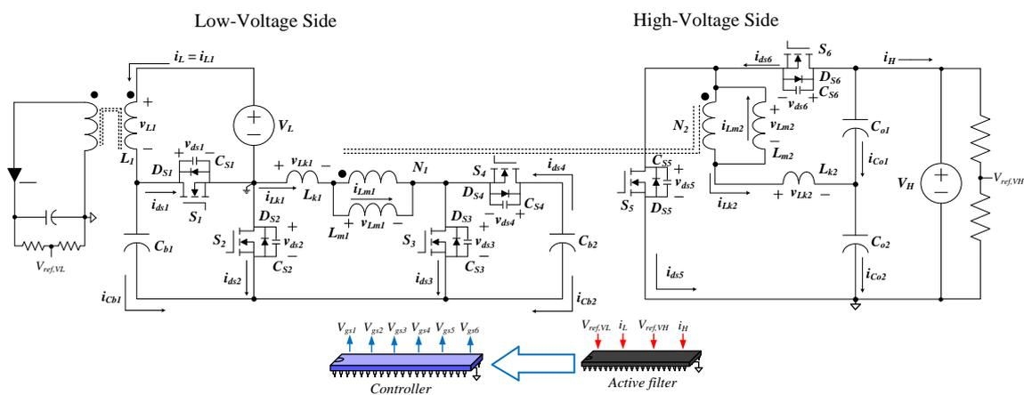
Figure 2. Schematic of the proposed bidirectional converter.
