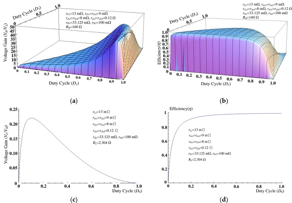
Figure 11. The relationships of voltage gain versus duty ratio and efficiency versus duty ratio while considering non-ideal effect: (a)  $M'_{step-up}$ ; (b)  $\eta_{step-up}$ ; (c)  $M'_{step-down}$ ; and (d)  $\eta_{step-down}$ .
