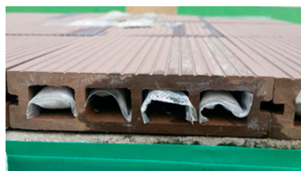
Figure 2. Packed PCM placed within the hollows of the wood-plastic composite (WPC) plate.
