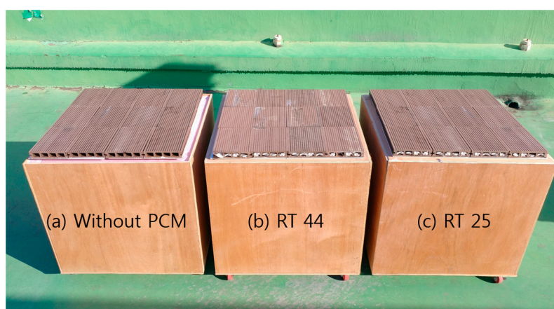
Figure 5. Small-scale models with as-manufactured WPC. (a) Without PCM; (b) Containing RT 44 in the hollows; and (c) With RT 25 in the hollows.
