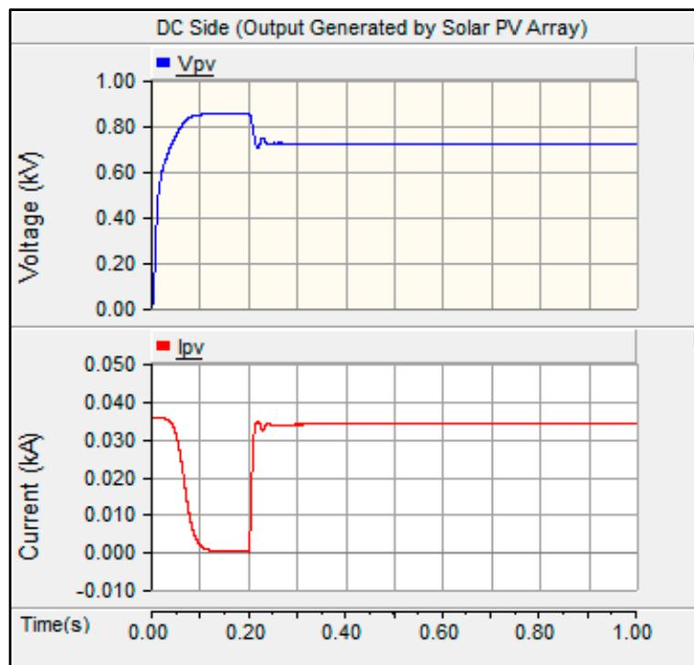
Figure 7. DC voltage and DC current.
