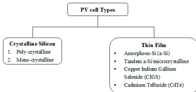
**Figure 1.** Photovoltaic (PV) cell types.
