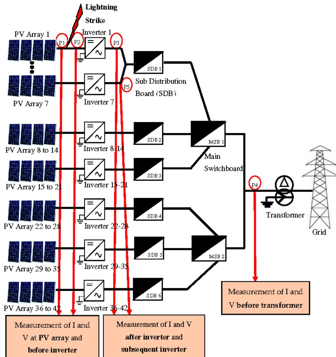
Figure 9. Strike points at Solar PV farm.
