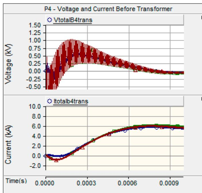
Figure 12. Transient voltage and current at P4 (transformer).
