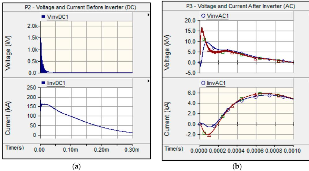
Figure 11. (a) Transient voltage and current at P2 (before inverter PV Array 1); (b) Transient voltage and current at P3 (after inverter PV Array 1).
