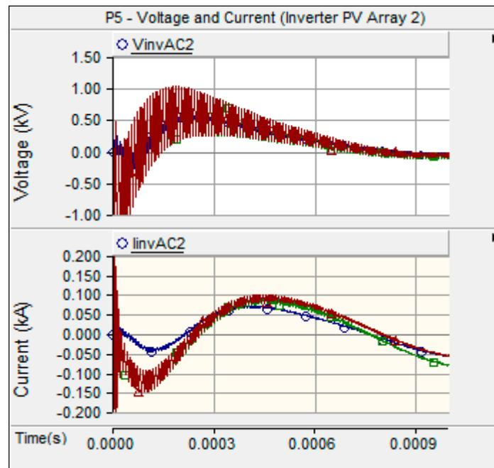
Figure 13. Transient voltage and current at P5 (inverter PV Array 2).
