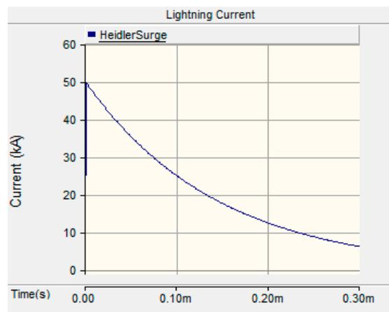
Figure 2. Lightning impulse current wave shape at 0.25/100  $\mu\text{s}$ .
