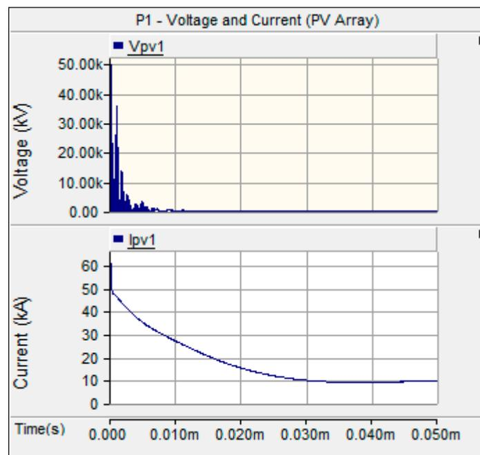
Figure 10. Transient voltage and current at P1 (solar PV Array 1).
