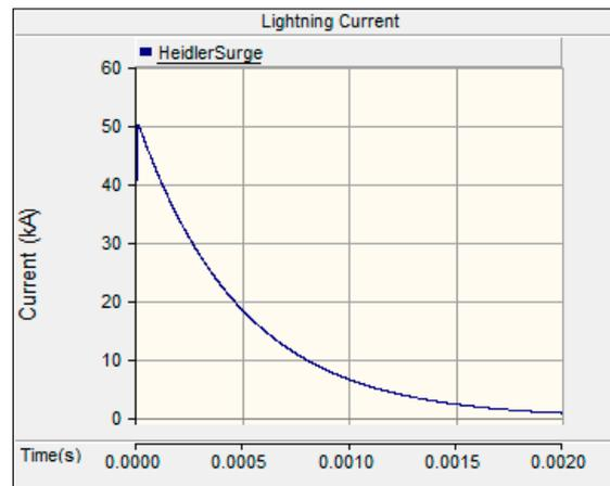
Figure 4. Lightning impulse current wave shape at 10/350  $\mu$ s.
