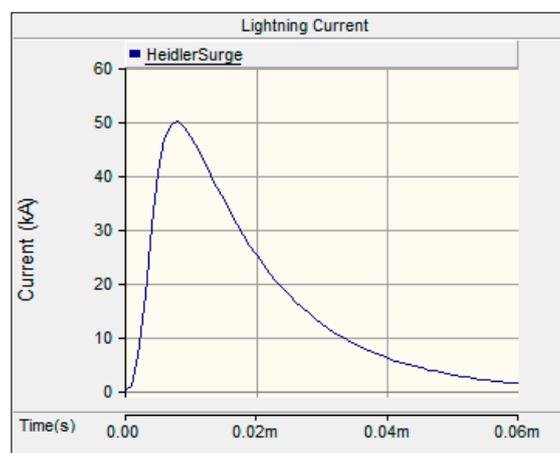
Figure 3. Lightning impulse current wave shape at 8/20  $\mu\text{s}$ .
