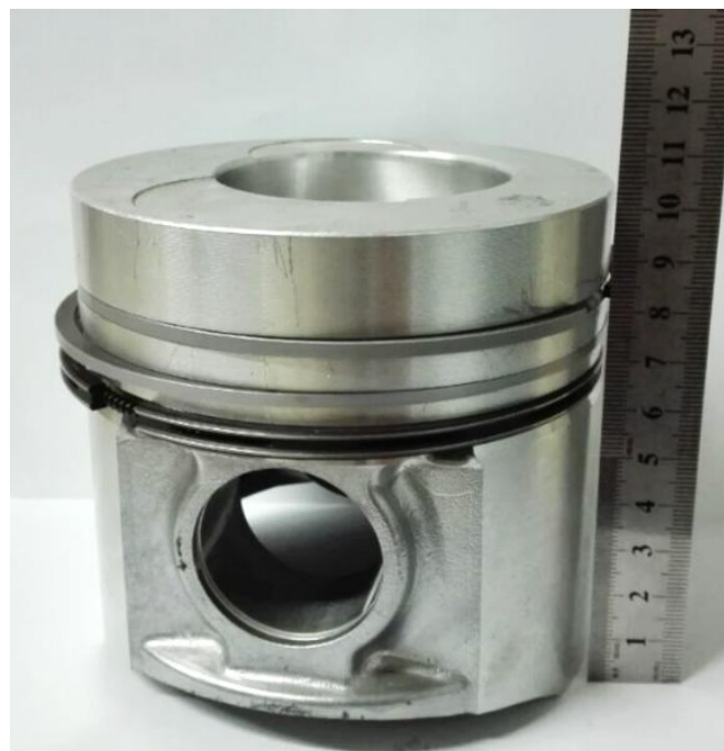
Figure 16. Configuration of piston rings.
